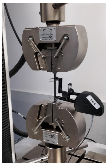
Figure 4.1: Experimental setup for tensile tests.
