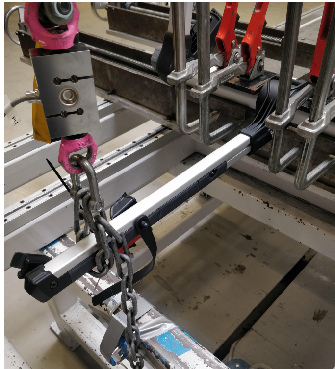
Figure 5.2: Experimental setup for mechanical testing of console.
