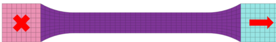
Figure 4.8: Setup of the tensile test simulation. The red cross indicates the fixed boundary condition and the red arrow indicates the displacement.
