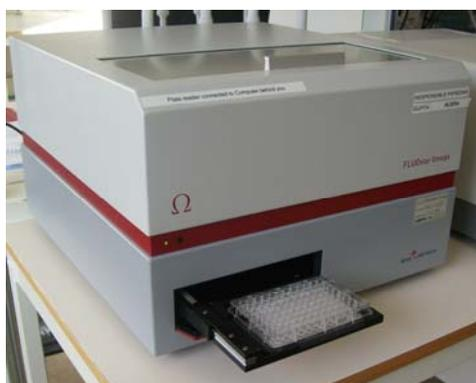
Figure 15 – Plate reader (*Fluostar Omega, BMG LabTech*).
