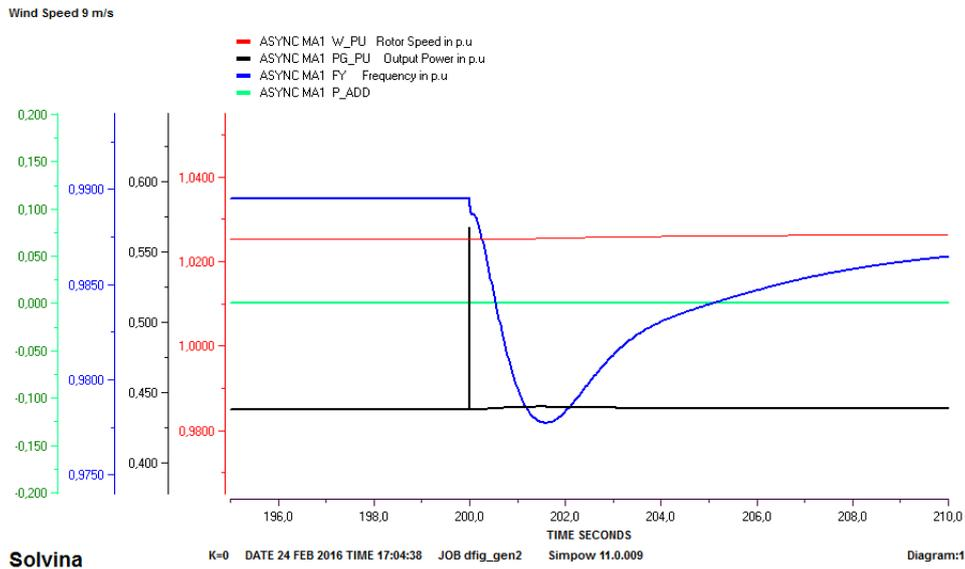
Figure 4.16: Output of the wind turbine in medium wind speed region with  $k=0$
