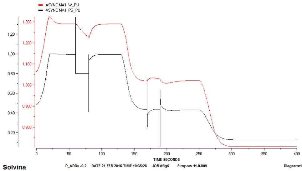
**Figure 4.5:** Output of the asynchronous machine at  $P\_ADD = -0.2$  p.u
