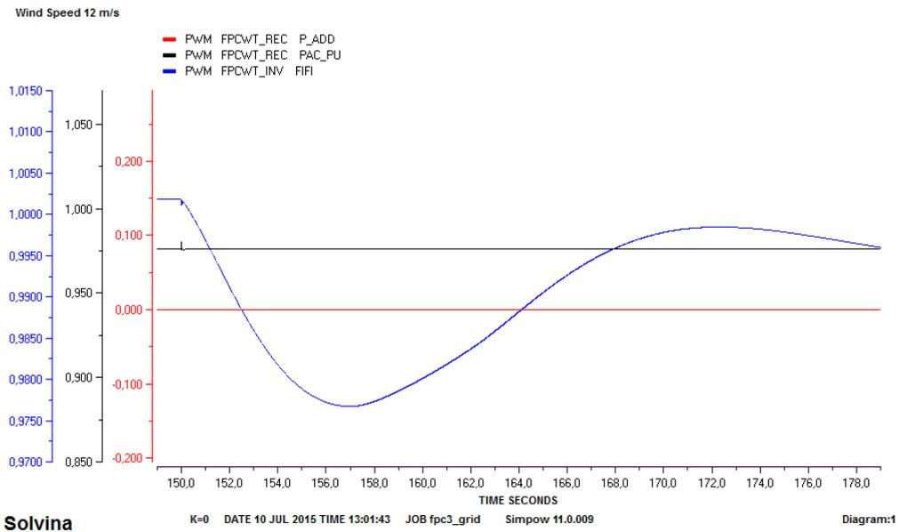
Figure 6.9: Frequency response with current rating 1.1 p.u and no synthetic inertia
