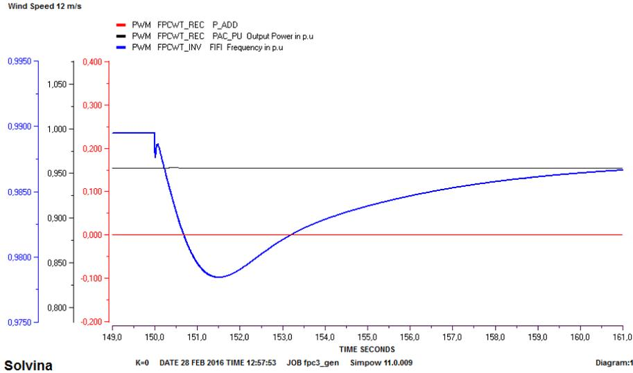
Figure 5.5: FPC output with no synthetic inertia included, i.e  $k=0$
