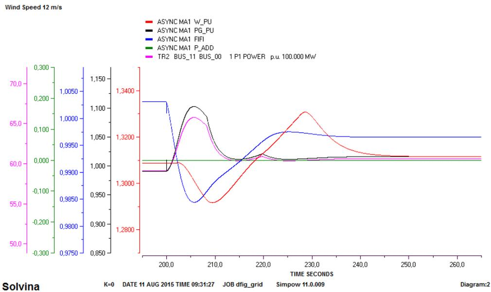
Figure 6.2: Frequency response of the network with no synthetic inertia
