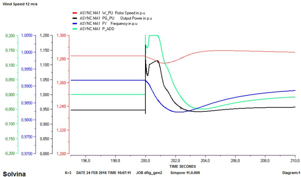
Figure 4.12: Output of wind turbine at high wind speed with  $k=3$
