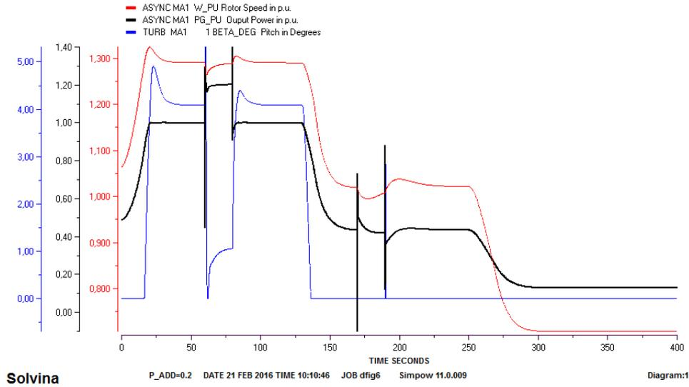
**Figure 4.4:** Output of asynchronous machine with  $P\_ADD = 0.2$  p.u applied in high and medium wind region
