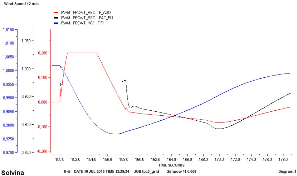
Figure 6.8: Frequency response with current rating 1.04 p.u and  $k=5$
