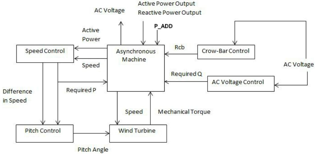
**Figure 3.2:** Block Diagram for Doubly Fed Induction Generator model
