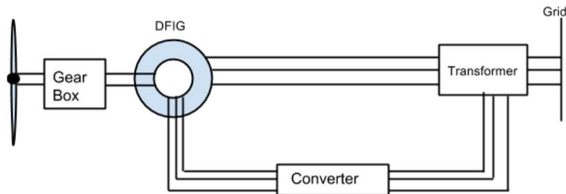
**Figure 3.1:** Doubly-fed Induction Generator Wind Turbine
