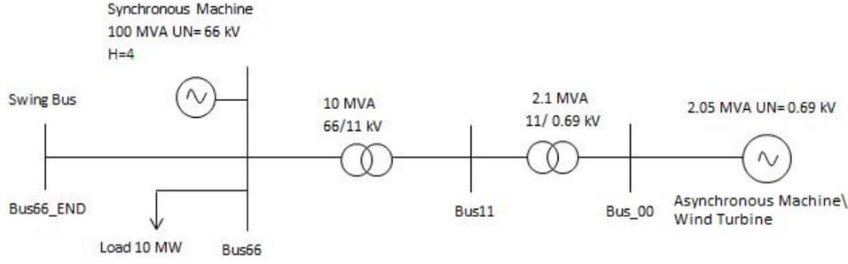
**Figure 4.7:** Single line diagram with the synchronous machine and load included
