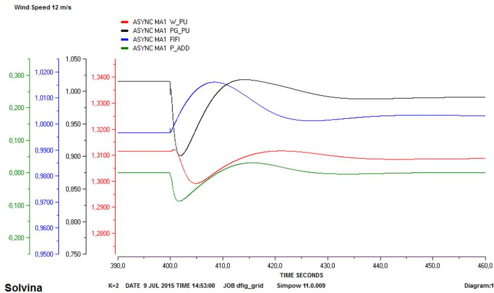
Figure 6.5: Frequency response of the network with synthetic inertia
