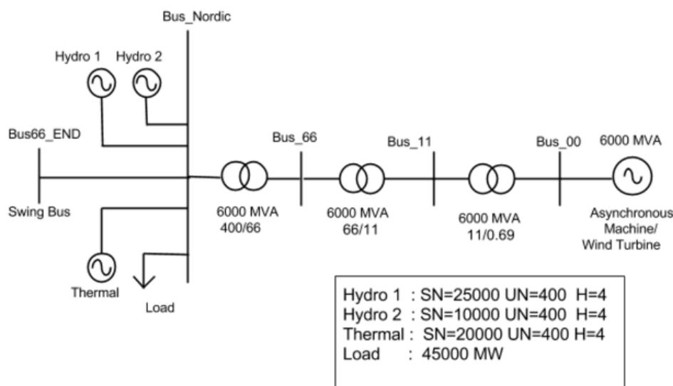
**Figure 6.1:** Single Line Diagram of the Nordic network with DFIG wind turbine
