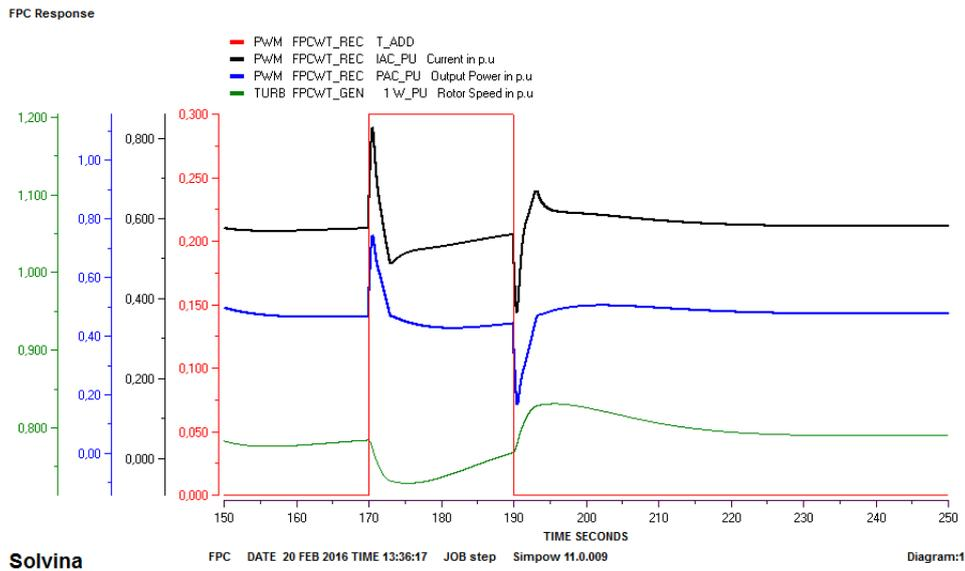
**Figure 5.3:** Step response for the FPC during medium wind speed with additional step of 0.2 p.u.
