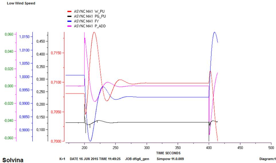
**Figure 4.11:** Wind turbine output at low wind speed condition with  $k=1$  which causes the system to become unstable.
