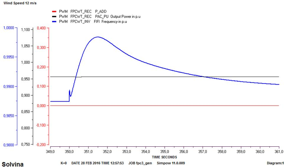
Figure 5.7: FPC output in case of over-frequency with  $k=0$
