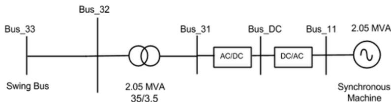
**Figure 5.1:** Single line diagram for FPC wind turbine
