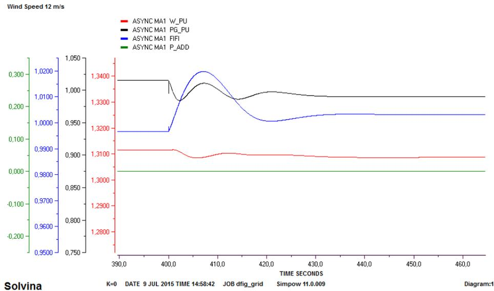
**Figure 6.4:** Frequency response of the network with no synthetic inertia
