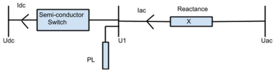
**Figure 3.6:** PWM converter model
