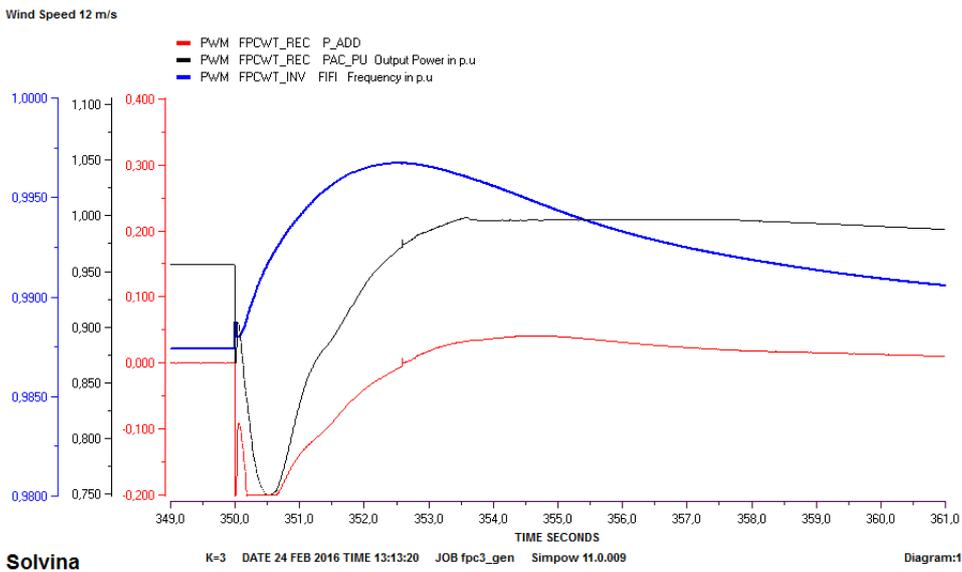
Figure 5.8: FPC output in case of over-frequency with  $k=3$
