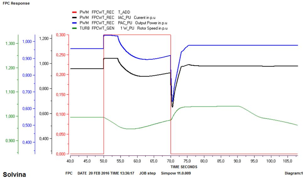
**Figure 5.2:** Step response for FPC during high wind speed with additional step of 0.2 p.u.
