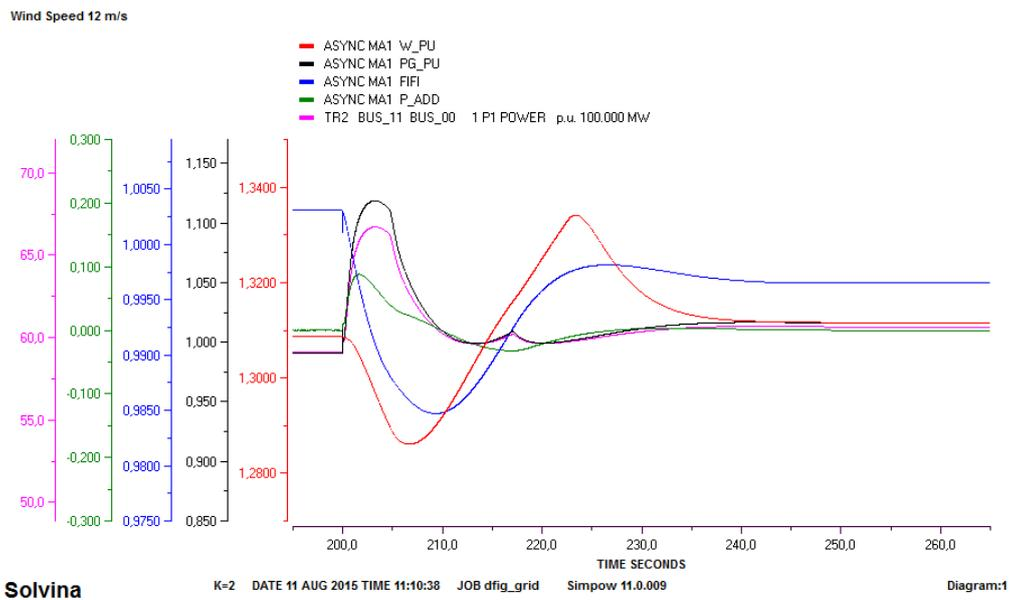
Figure 6.3: Frequency response of the network with synthetic inertia.  $K=2$
