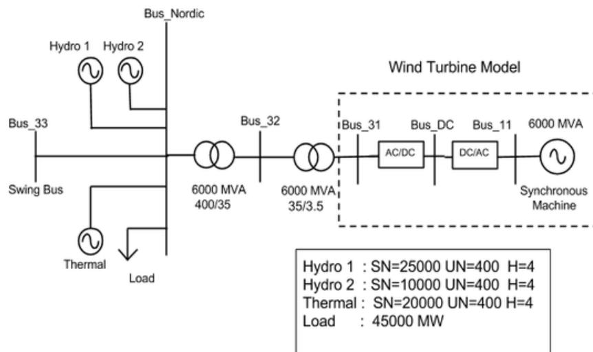
Figure 6.6: Single line diagram of the Nordic network with FPC wind turbines
