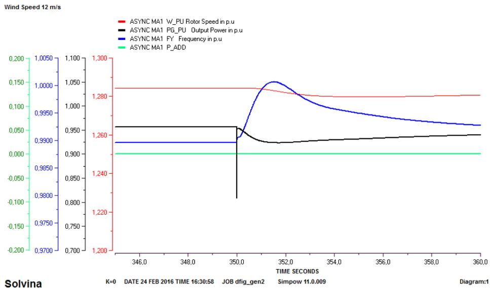
**Figure 4.14:** Output of the wind turbine in high wind speed in case of over-frequency with  $k=0$
