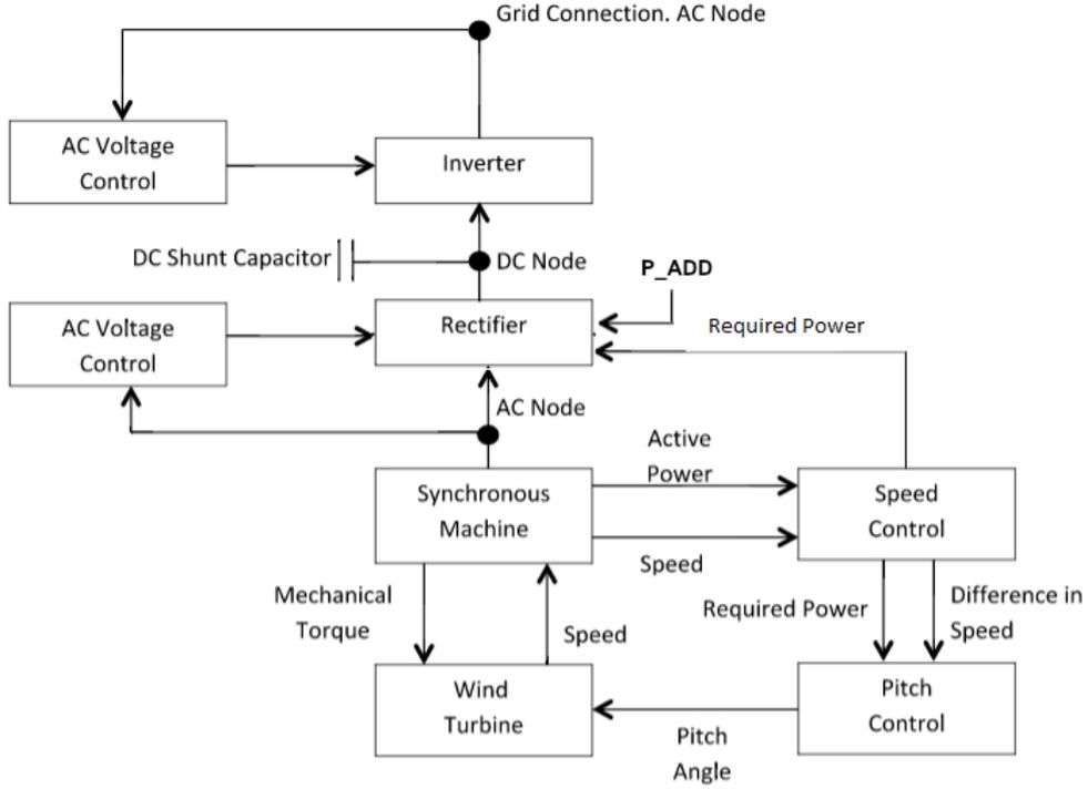
**Figure 3.5:** Block Diagram for Full Power Converter Wind Turbine Model
