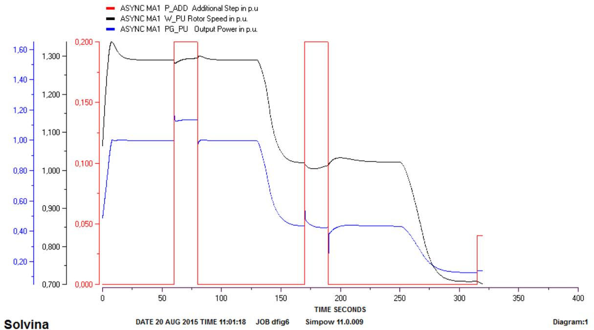
**Figure 4.6:** Stalling of simulation for the DFIG wind turbine at low wind speed with  $P\_ADD = 0.04$  p.u.
