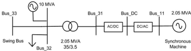
**Figure 5.4:** Modified single line diagram
