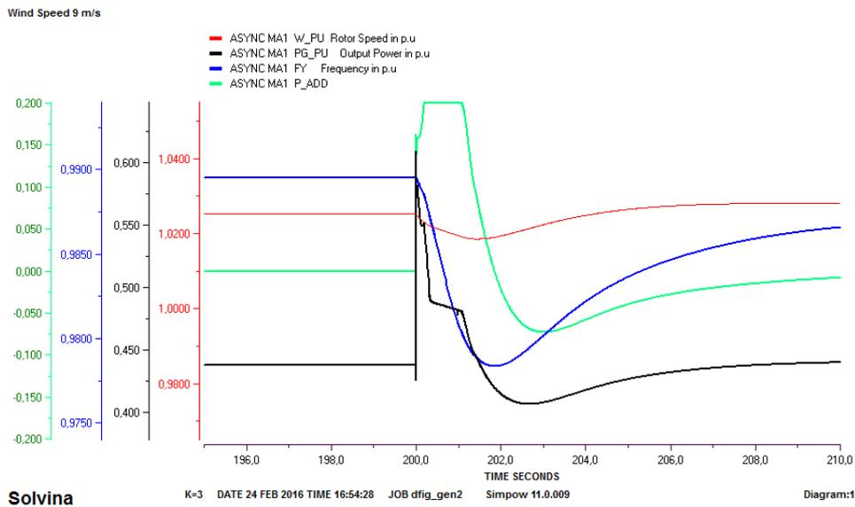
Figure 4.17: Output of the wind turbine in medium wind speed with  $k=3$
