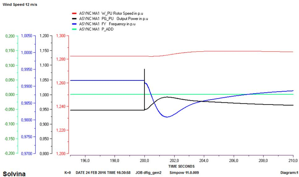
Figure 4.13: Output of the wind turbine at high wind speed with  $k=0$
