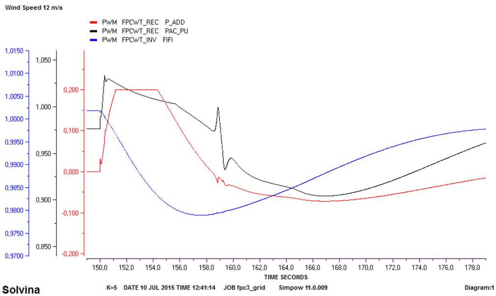
Figure 6.10: Frequency response with current rating 1.1 p.u and  $k=5$
