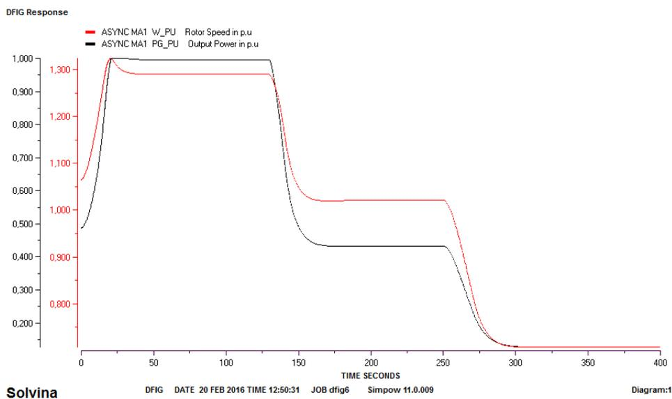
**Figure 4.3:** Rotor speed and output power of the wind turbine for the given wind profile
