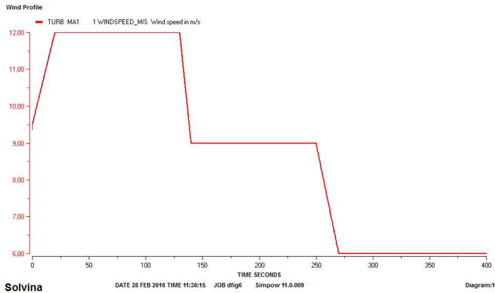
**Figure 4.2:** Wind Profile Used for Simulations
