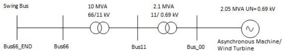
**Figure 4.1:** Single line diagram for the wind turbine
