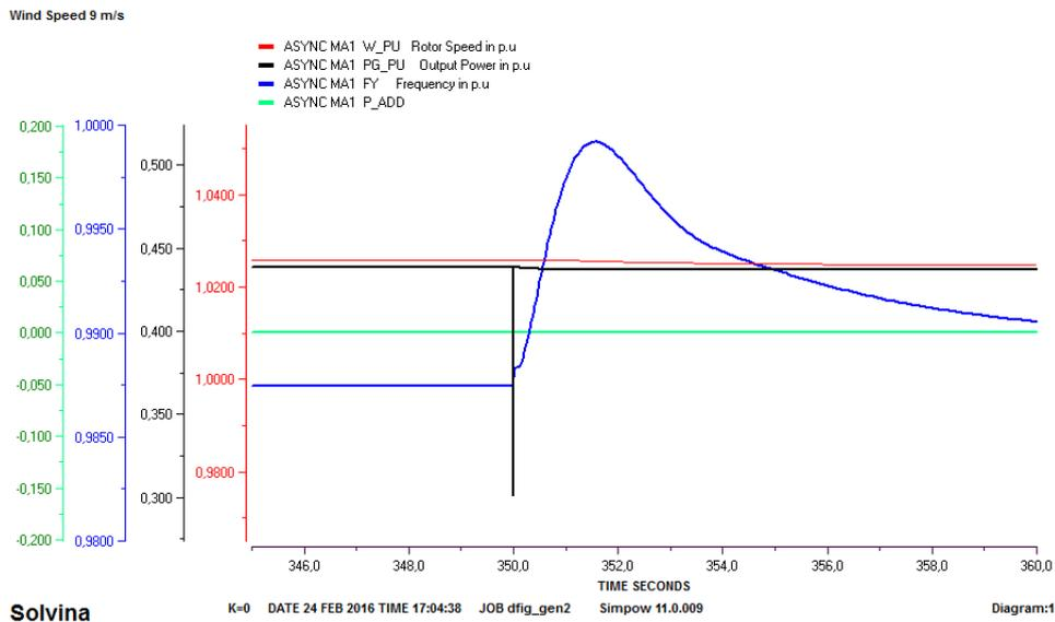
**Figure 4.18:** Output of the wind turbine in medium wind speed in case of over-frequency with  $k=0$
