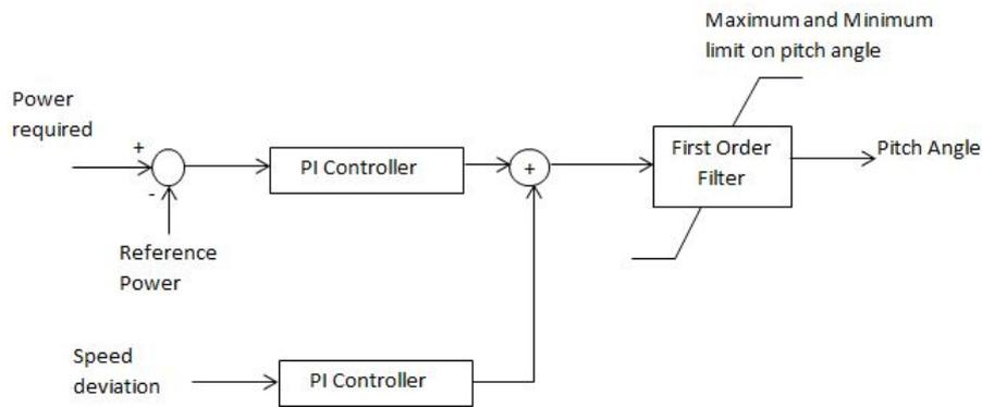
**Figure 3.4:** Block Diagram of Pitch Control Model
