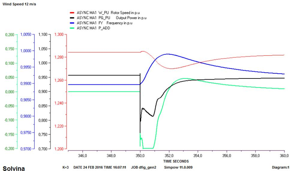
**Figure 4.15:** Output of the wind turbine in high wind speed in case of over-frequency with  $k=3$
