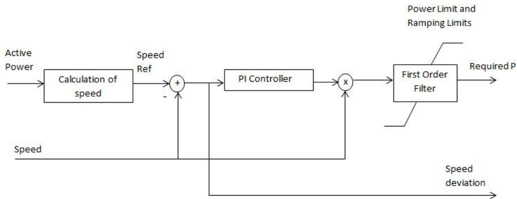
**Figure 3.3:** Block Diagram of Speed Control Model
