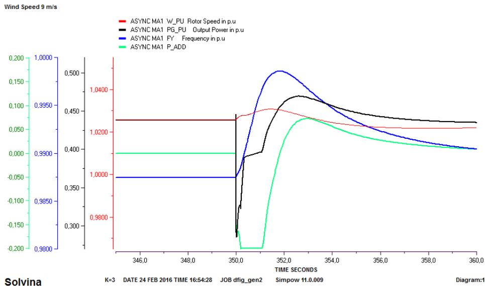
**Figure 4.19:** Output of the wind turbine in medium wind speed in case of over-frequency with  $k=3$
