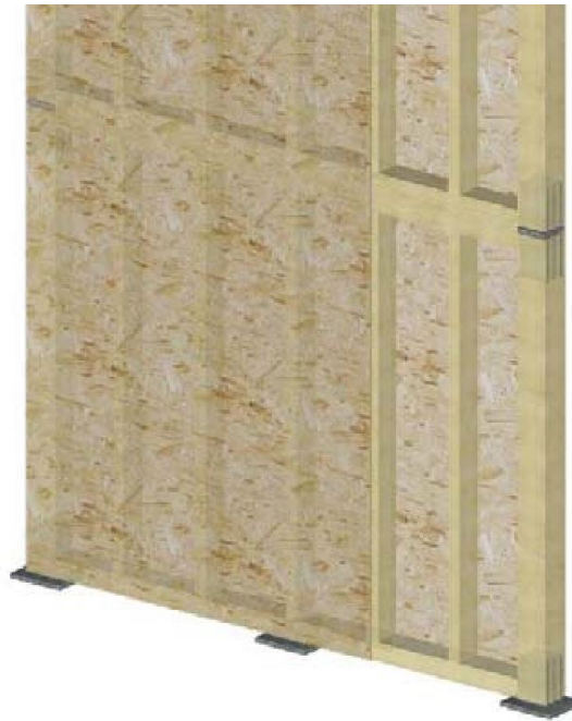
Figure 5.8: Alternative timber frame shear wall construction with cut sill plates and vertically connected studs, Jung (2013).
