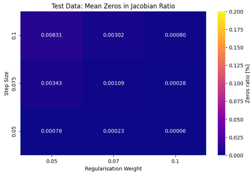
Figure 4.14: Heatmap of mean zeros in Jacobian ratio, with pyramid (1,6), 10 iterations and affine transformation in pre-registration.
