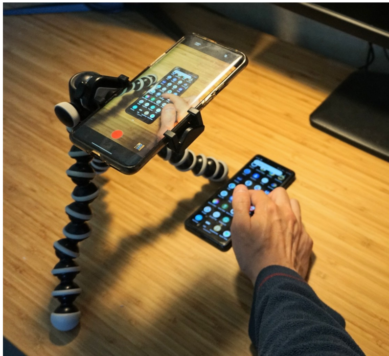
Figure 7.3: The end-to-end latency test setup, filming different devices using a tripod mounted smartphone capable of 240fps video.
