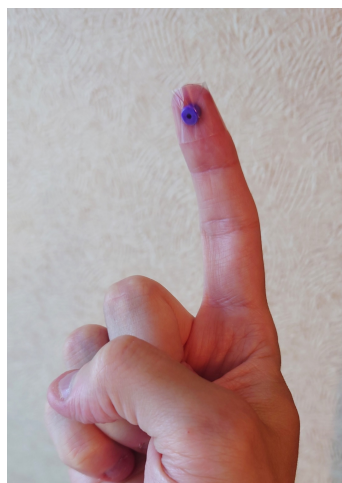
Figure 7.5: The plastic piece placed on the finger during the demonstrations of the test applications for achieving more reliable touch input.
