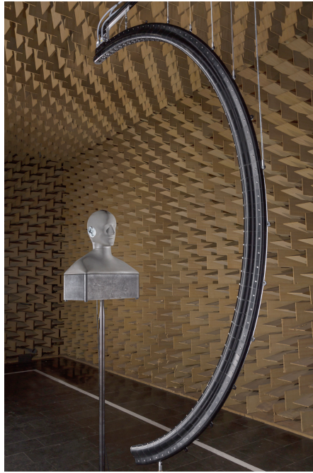
Figure 1.1: Dummy head HRTF measurements in anechoic chamber, RWTH Aachen University
