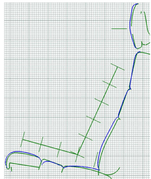
Figure 22. Intended design (green lines) compared with a scanned seat (blue lines).
