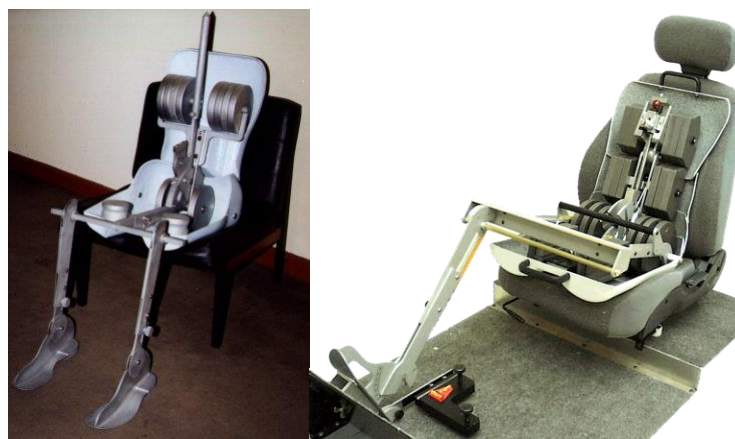
Figure 6. Devices for measuring H-point, from SAE J826 and J4002
