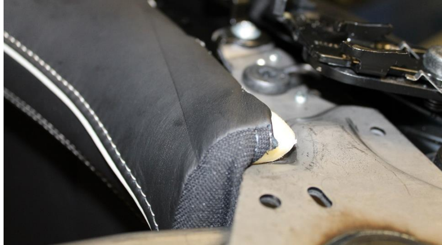
Figure 11. Picture of foam and trim from tear down.
