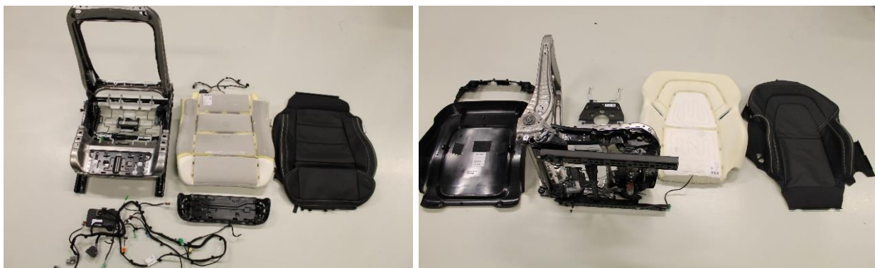
Figure 12. Seat components in cushion and back affecting H-point.
