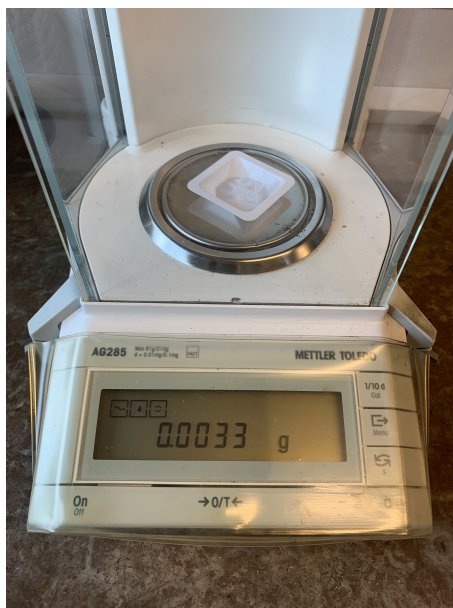
Figure 3.2: Sensitive scale used to weigh the fibres.
