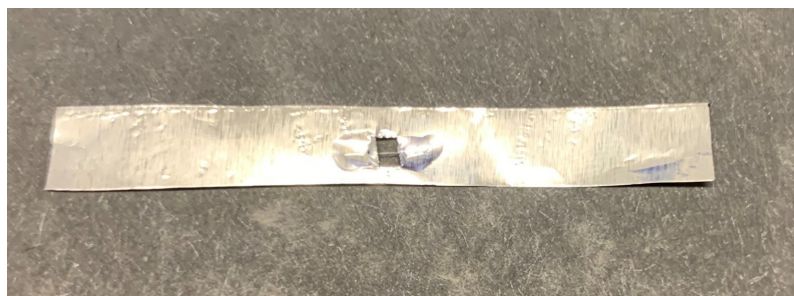
Figure 3.7: Illustration of an aluminum frame with the fibre glued on.
