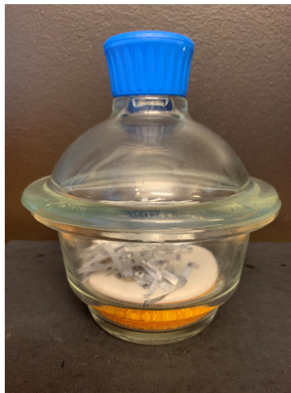
Figure 3.10: Illustration of the desiccator used throughout this thesis.
