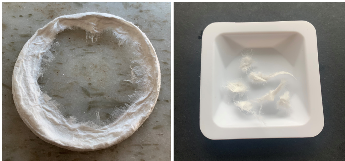
Figure 3.1: Fibre cake of mesh 14 from Tetra Pak to the left and collected fibres on the plate to the right.
