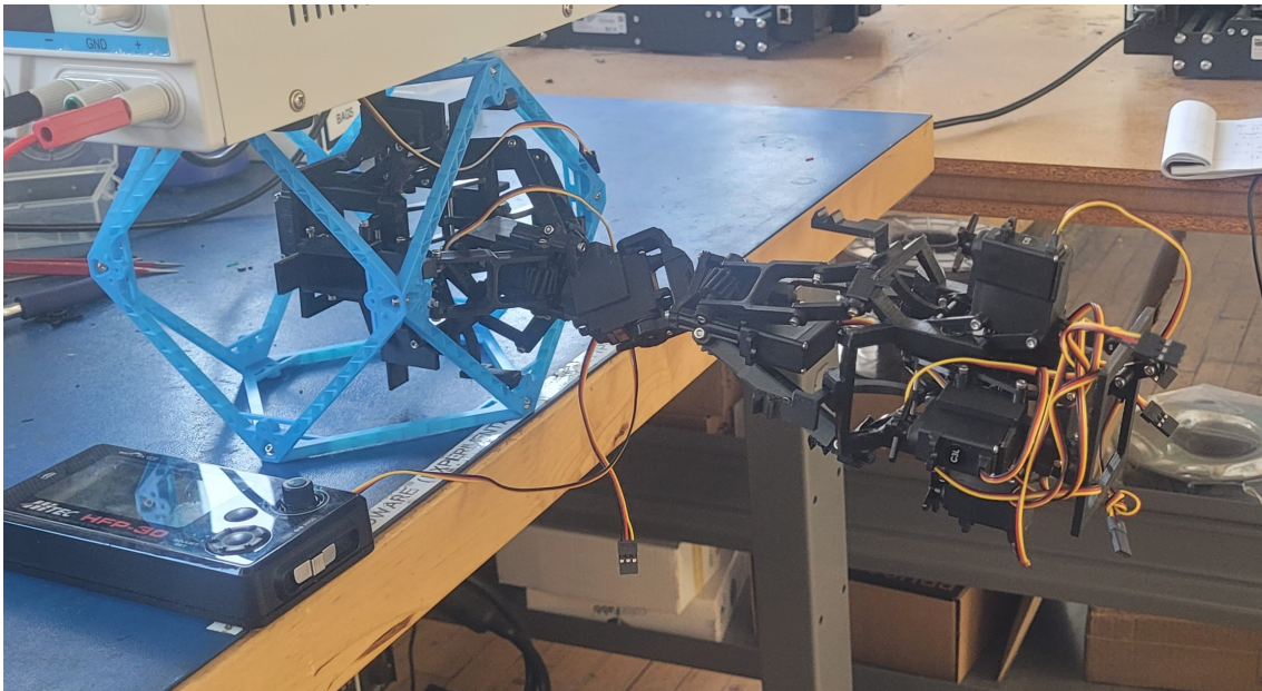
Figure 4.5: mMMIC-I is attached to a voxel phase and shows that it is capable of lifting itself to a horizontal position. This position was used to measure the hip functionality, as well as flex in the arm and gripper modules.
