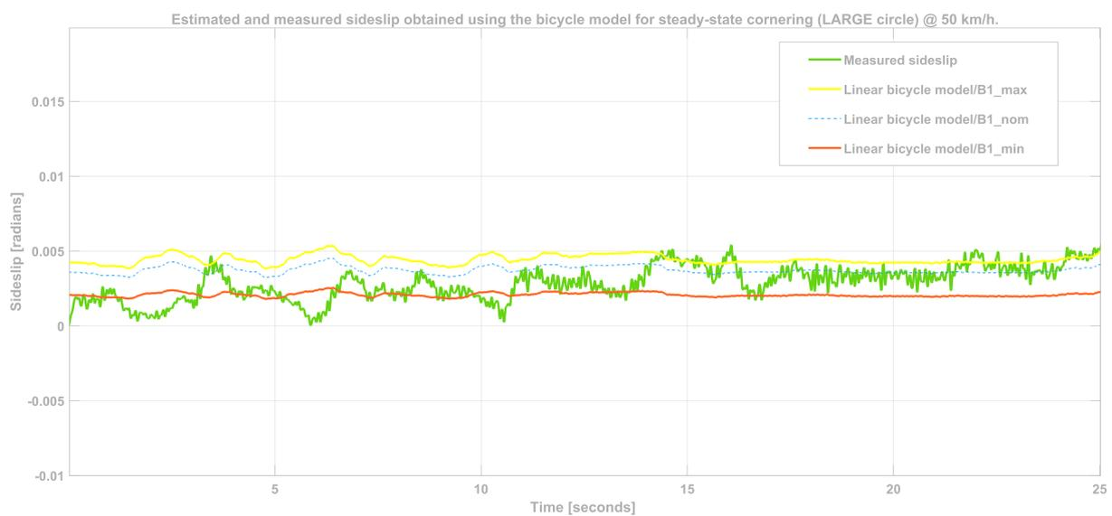
Figure 7.6: Estimated side-slip versus measured value using bicycle model for steady state cornering with large radius.
