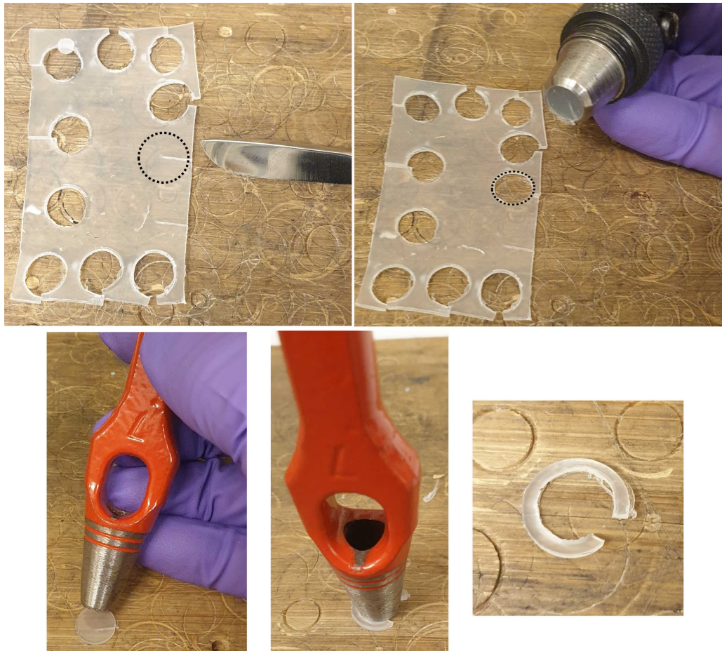
Figure A.2. The process of punching the PP spacers. See text for explanation.
