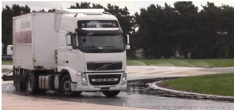
Figure 1.2: *Test vehicle (fitted with FABVs) carrying out brake-in-turn test on wet basalt surface.*
