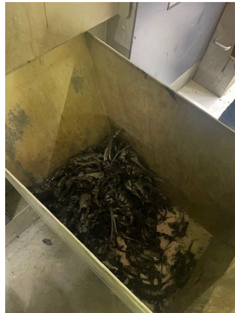
Figure 2.5: The extruded contamination by the erema machine
