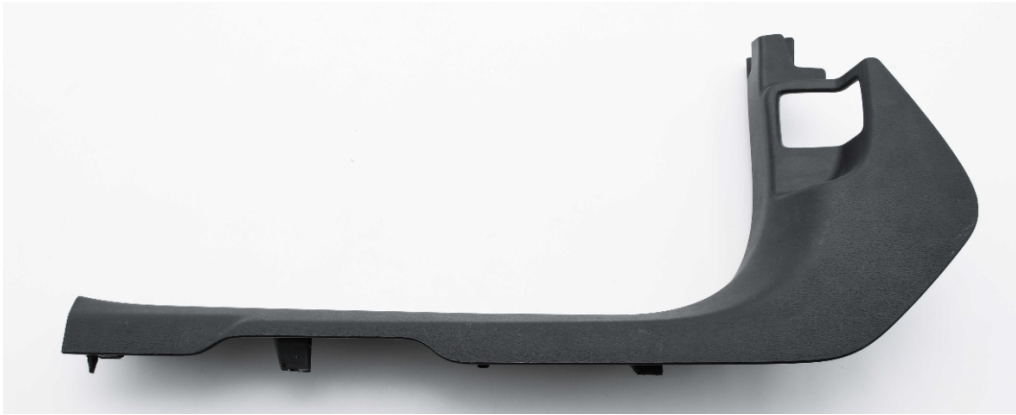
Figure 1.2: Close-up of one of the hard trim panels, the threshold
