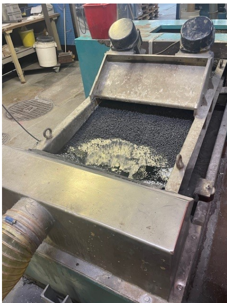
Figure 2.6: The granules created by the erema machine
