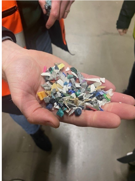
Figure 2.3: The shredded PCR PP that arrives to Rondo
