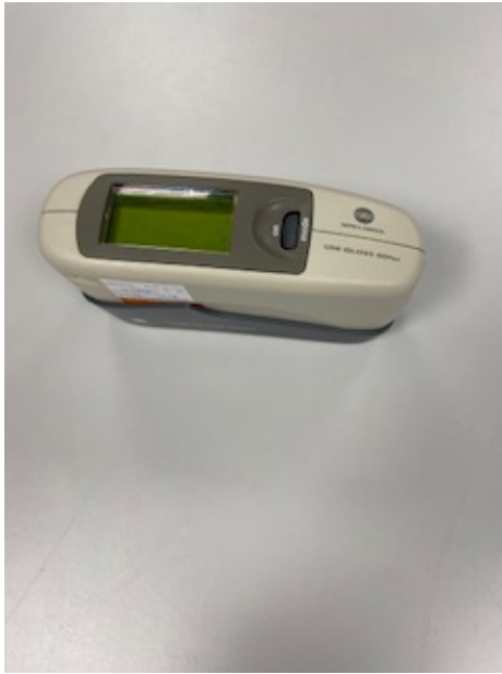
Figure 3.30: The Glossmeter tool
