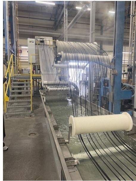
Figure 2.9: The spaghetti-like strings drying and on their way to be cut into granules
