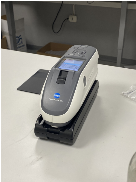
Figure 3.27: The Spectrophotometer tool used to measure the color of the material
