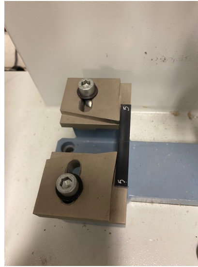
Figure 3.13: A sample ready for impact testing in the machine
