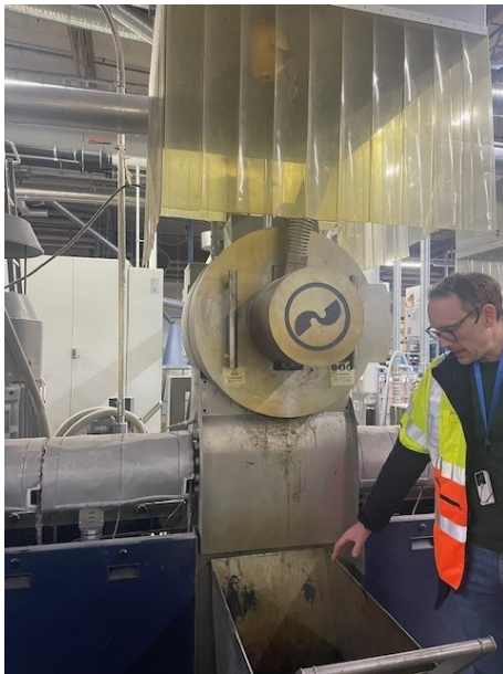
Figure 2.4: The erema extruder machine that removes contamination
