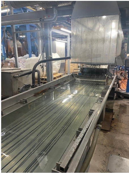
Figure 2.8: The spaghetti-like strings cooling down in water right after being extruded
