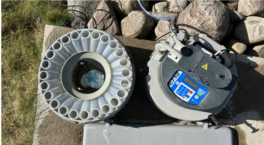
Figure 3.4: Opened ISCO-sampler, stacked with 24 bottles.
