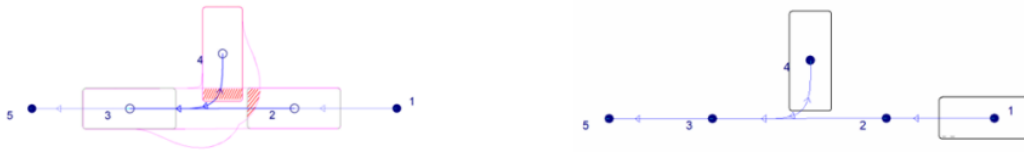
Figure 2.2: Illustration of a traffic rule: On the left, two vehicles risk colliding due to unrestricted movement. On the right, a traffic rule is applied that blocks segment (2,3) when a vehicle occupies point 4. This rule successfully prevents the collision by prohibiting access to segment (2,3).
