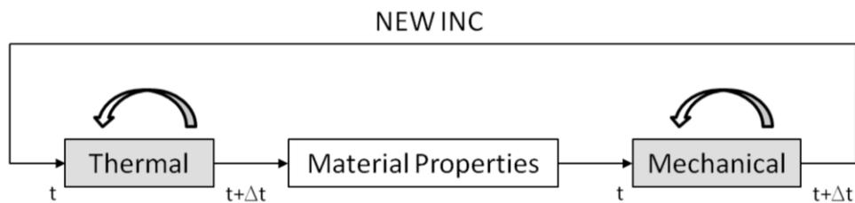
Figure 2.6 Overview of flow in a TM analysis, (Mattsson, 2015)
