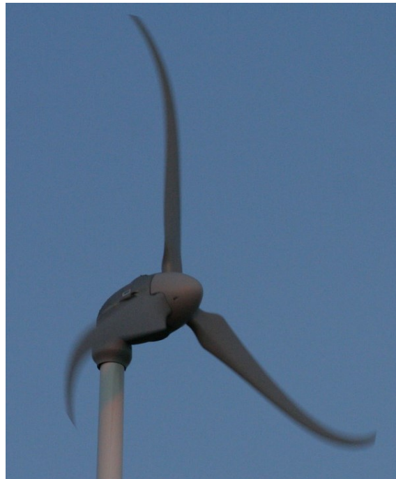
Figure 3.2: Spatial distortion of a windmill caused by rolling shutter method [2]
