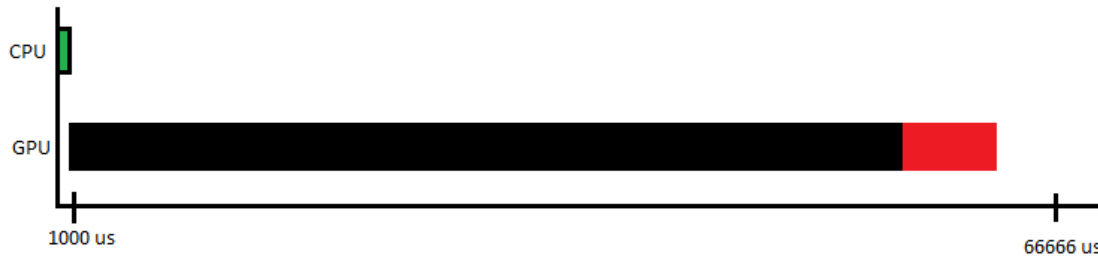
Figure 5.5: Schedule of a worst case cycle of the system. Green = Camera interface, Black = Yolo and red = Rendering.
