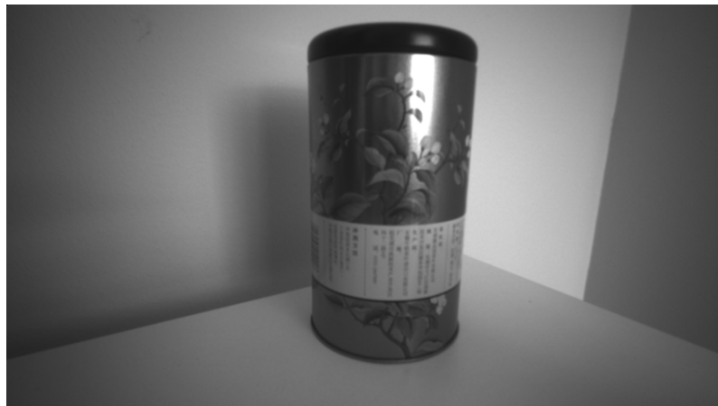
Figure 3.4: IR image of a tea jar in the dark with exposure time of 0.165 seconds, no extra illumination support.
