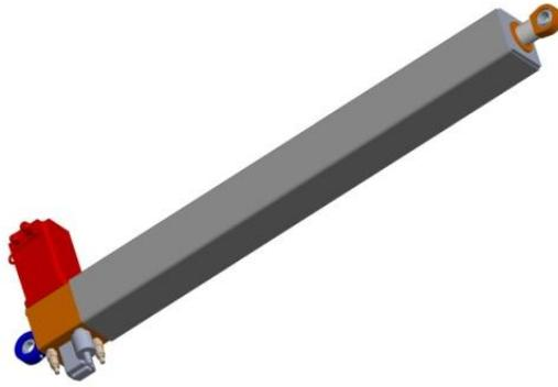
Figure 37. Standalone illustration of electro-hydraulic cylinder
