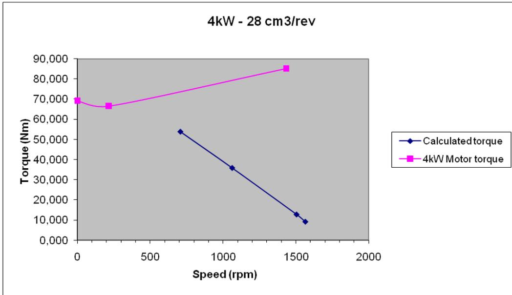
Figure 24. Example of torque curve with a 4 kW motor and a 28 cm<sup>3</sup>/rev displacement pump, calculated torque is the required torque at different rpm and the upper line illustrates the motor characteristics.
