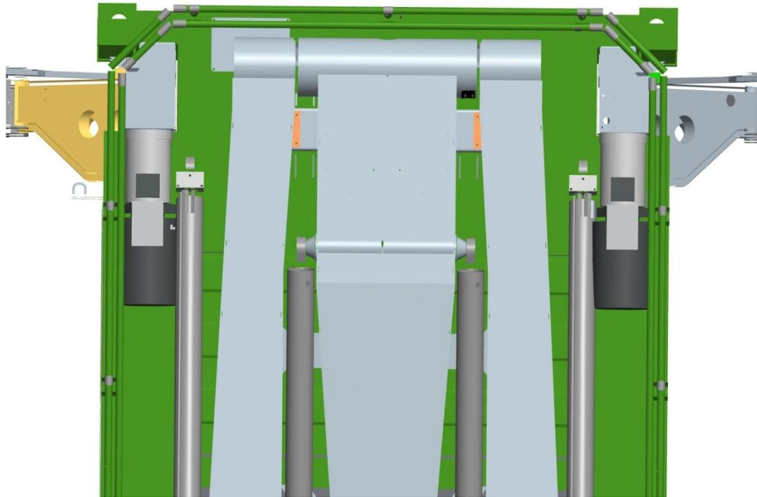
Figure 43. Mast power units, positioned on roof sides. No major interferences.
