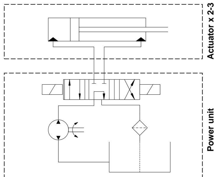
Figure 30. Generalization of the PowerPack configuration with a separate modular unit divided from the actuator.
