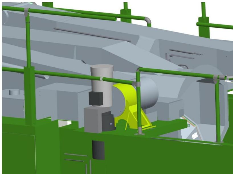
Figure 48. Close-up of an example with rear support leg power pack positioned as in the front; Interference with mast joint. Not a possible positioning in existing GAMB.
