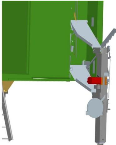
Figure 38. Close up of support leg EHC
