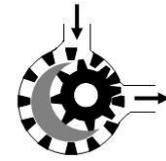
Figure 7. Internal gear pump
