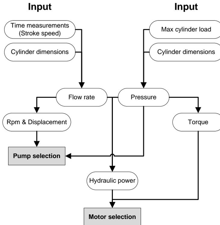
Figure 20. Method of calculation; Input is stroke speed, cylinder load and cylinder dimensions
