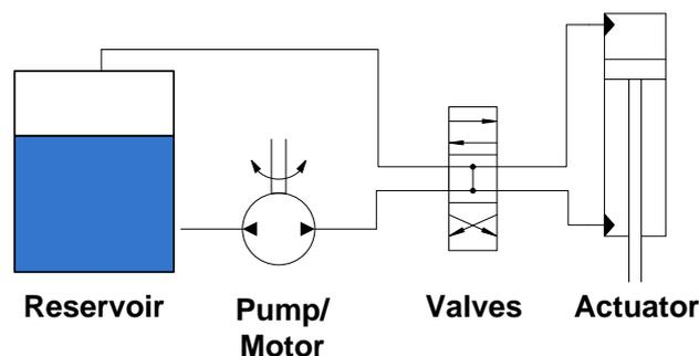
Figure 1. A generalization of how a hydraulic system can be conducted, with the main components included.
