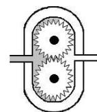
Figure 6. External gear pump
