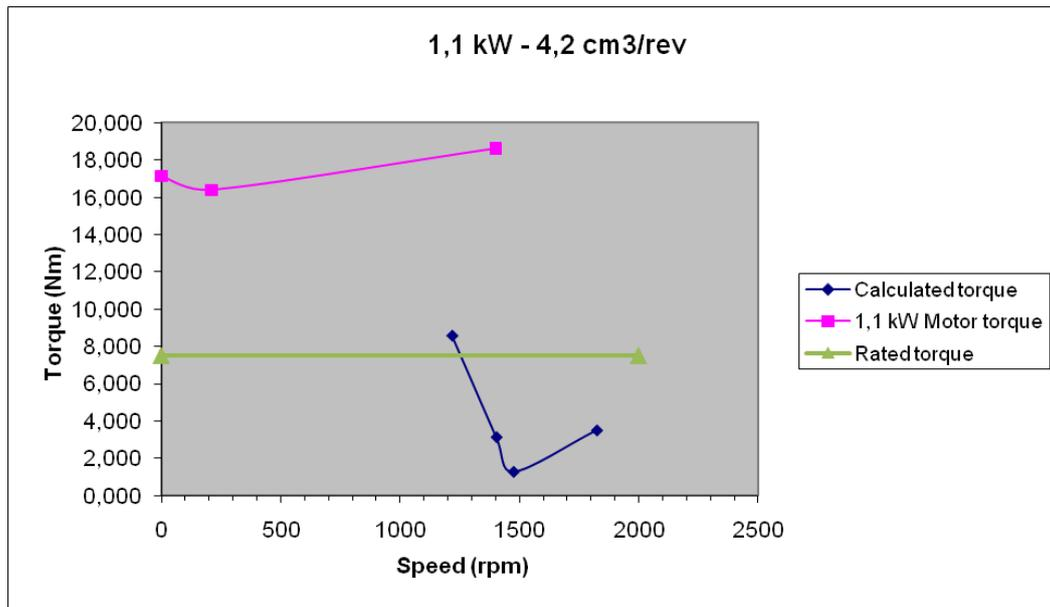
Figure 26. Example of a torque curve with a 1.1 kW motor and 4.2 cm<sup>3</sup>/rev displacement pump, including rated torque of the motor
