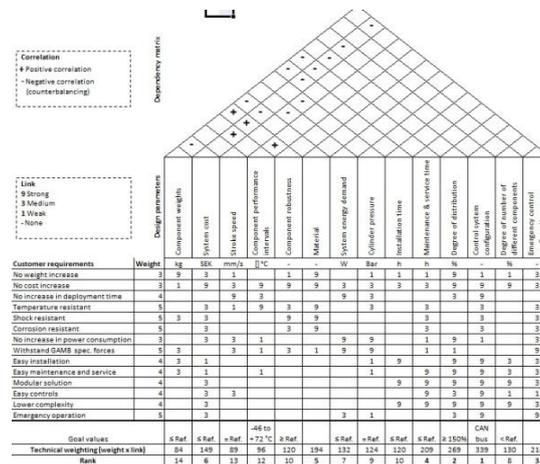
Figure 12. The "House of quality" matrix to translate customer requirements into design parameters
