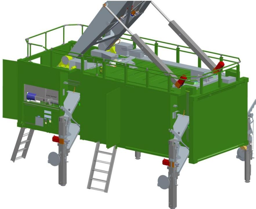
Figure 35. Overview of positions for electro-hydraulic cylinders in concept EHC
