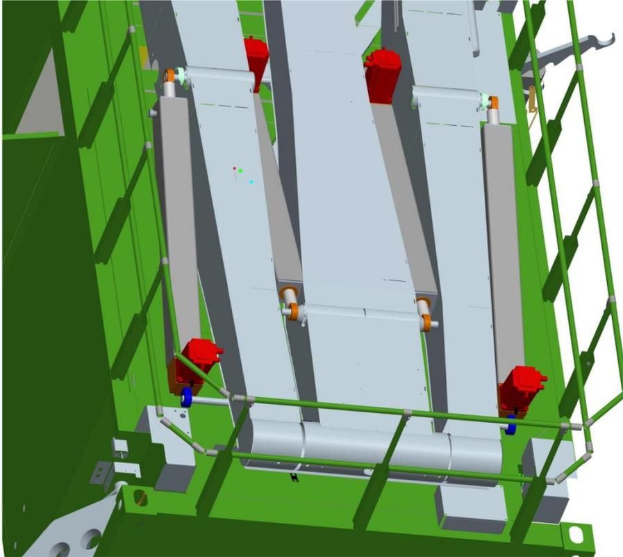
Figure 40. EHC with folded mast. Outer cylinders interfere with roof and inner cylinders interfere with the wide section of the upper mast section.
