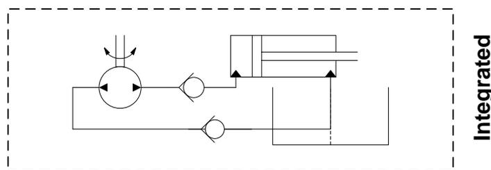
Figure 32. Generalization of the integrated EHC hydraulic circuit with basic components.
