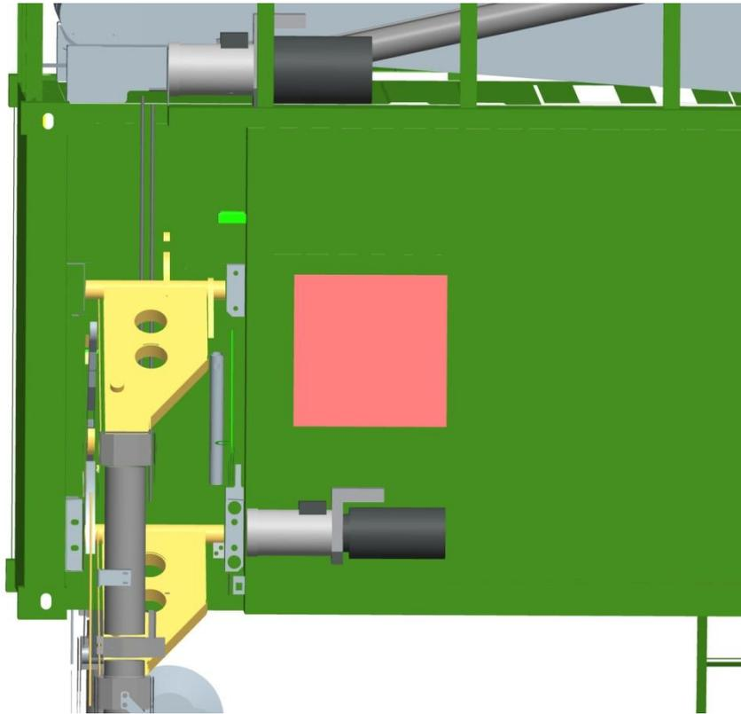
Figure 47. Alternative positioning of support leg power pack; Shelter rear end; Positioning horizontal/vertical outside leg compartment due to interference of mast joint.
