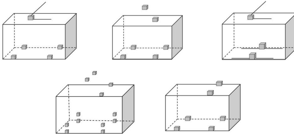
Figure 23. Examples of different distribution alternatives, a square represents a power unit.
