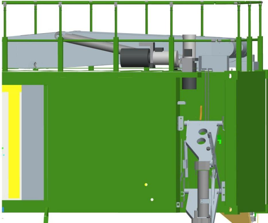
Figure 45. Example of support leg power unit position, above support leg; Shelter front. Compartment needs modification.
