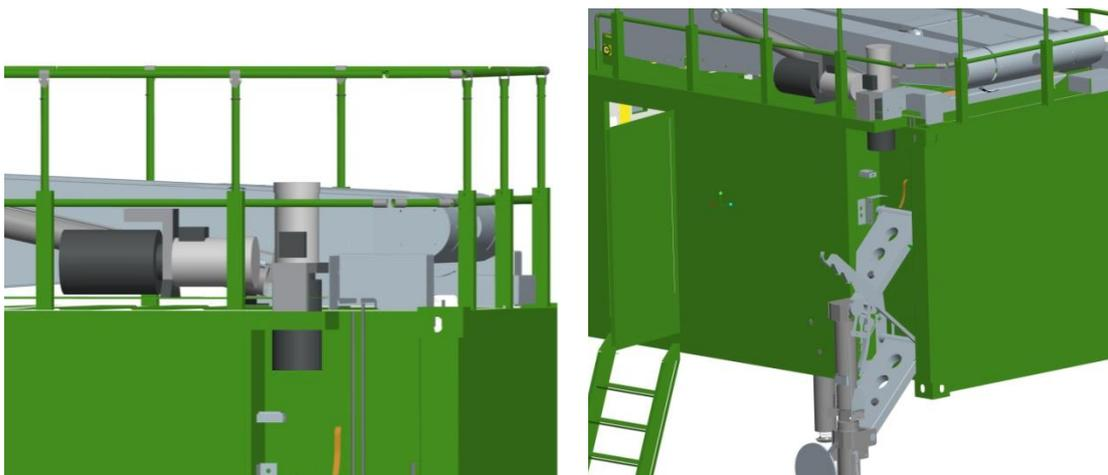
Figure 46. Various views of shelter front power packs, proposed positions.
