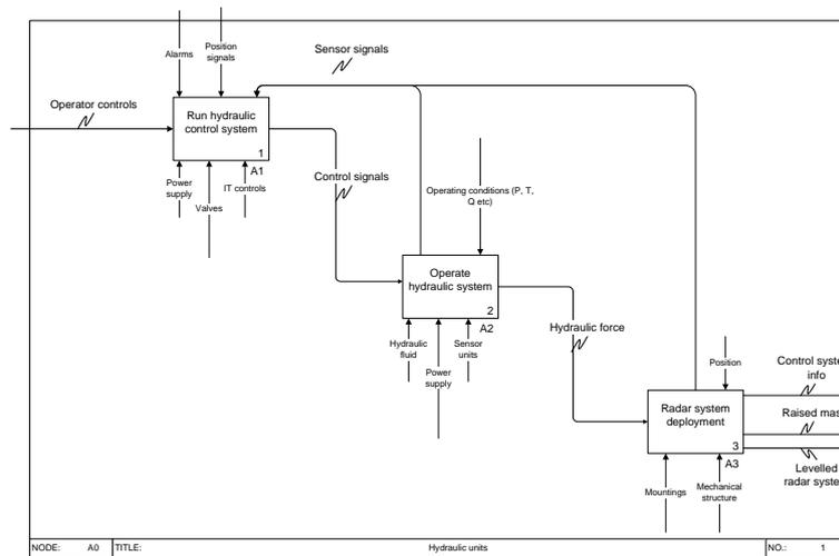
Figure 11. Illustration of an Idef0 process description
