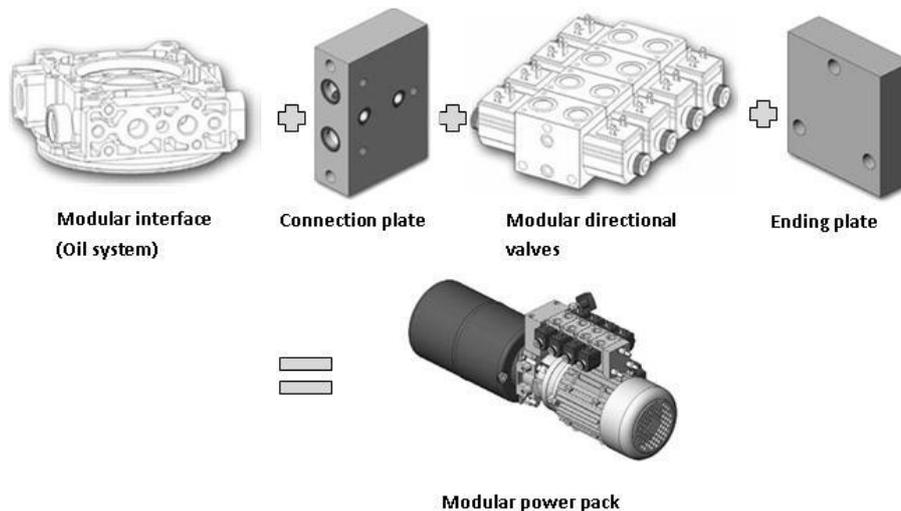
Figure 21. Illustration of power pack modularity
