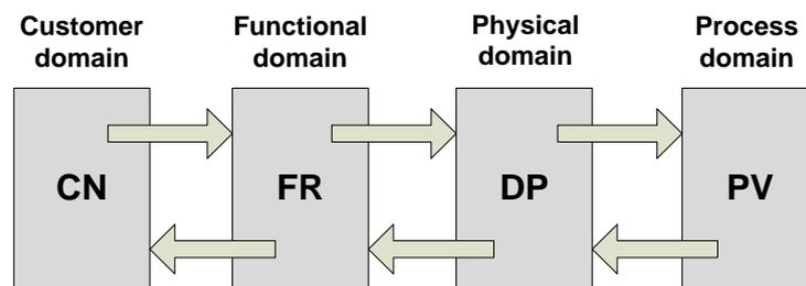
Figure 15. Mapping (“zig-zagging”) between domains according to axiomatic design methodology
