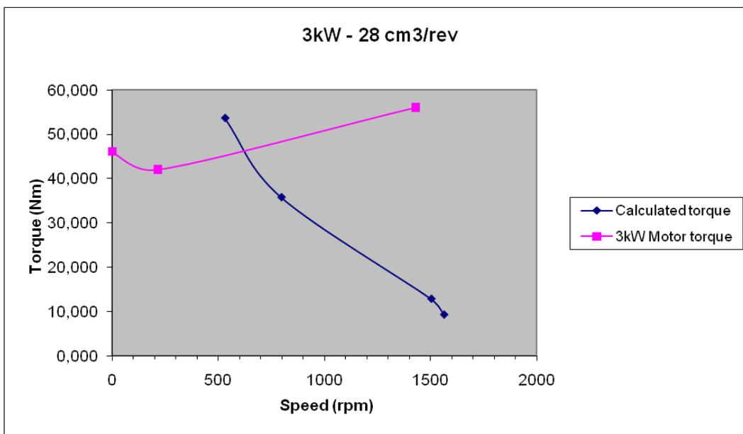
Figure 25. Example of a not acceptable torque curve with a 3 kW motor and a 28 cm<sup>3</sup>/rev displacement pump
