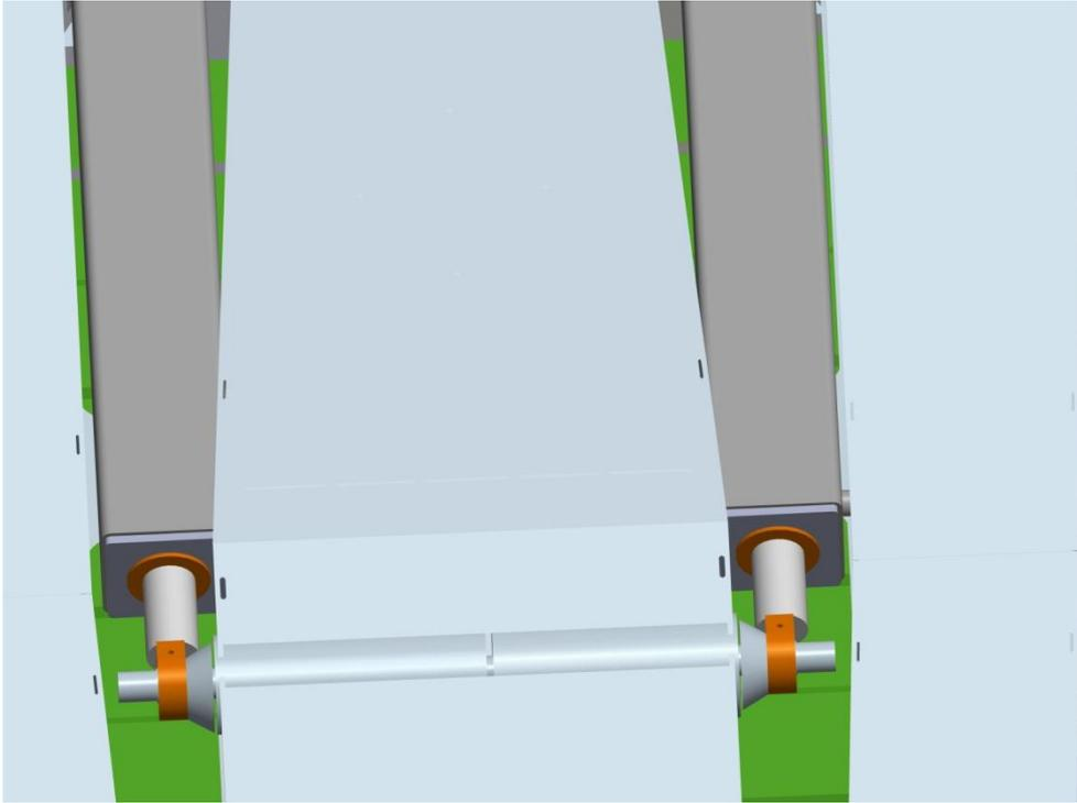
Figure 42. Close-up of upper mast cylinders that interfere with the upper mast section when folded.
