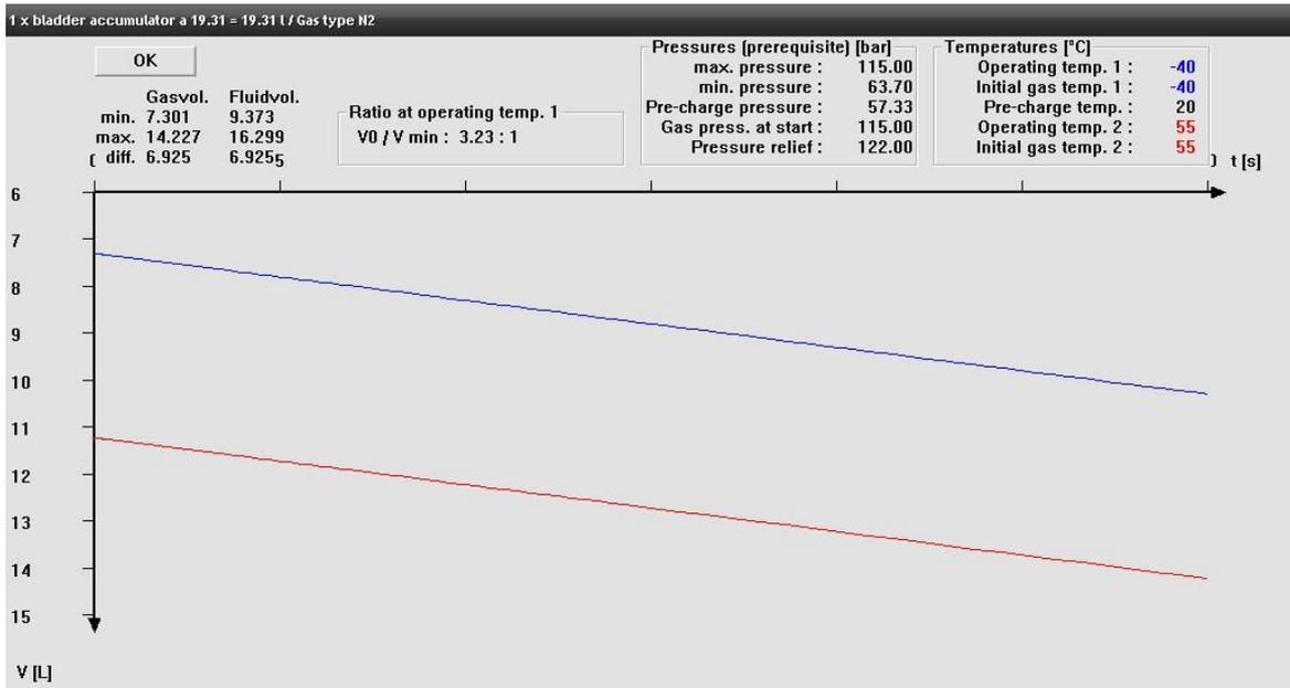
Figure 28. Result of temperature impact of accumulator volume from simulation
