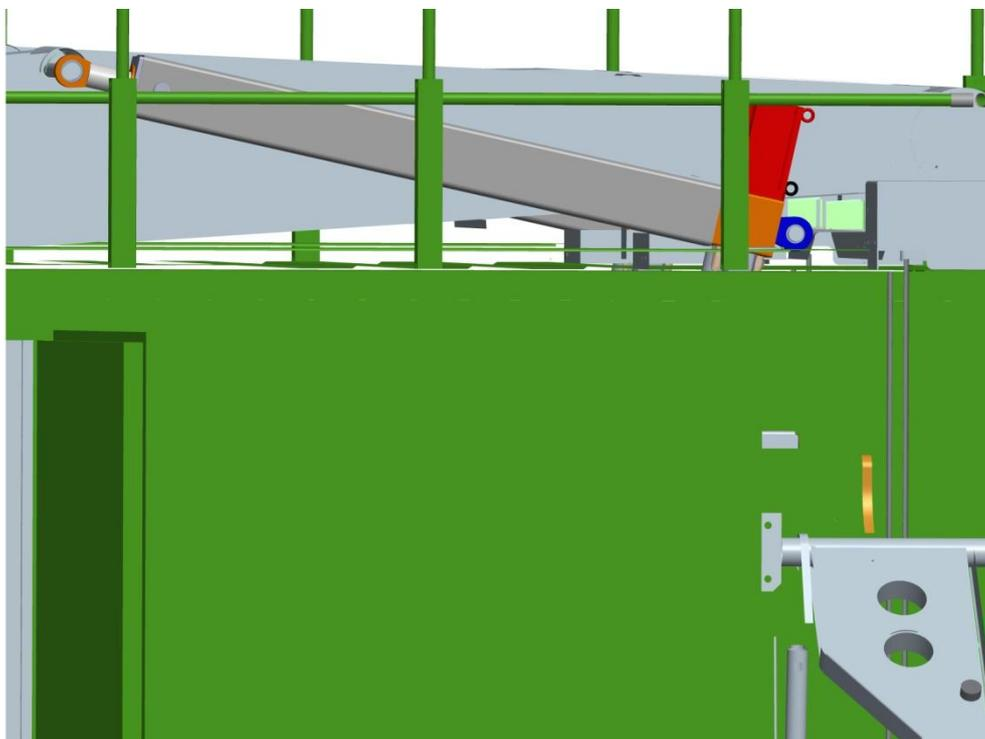
Figure 41. Close-up on lower mast cylinders with interfering pump and valves on the roof.
