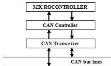
Figure 22. Illustration of a CAN bus structure
