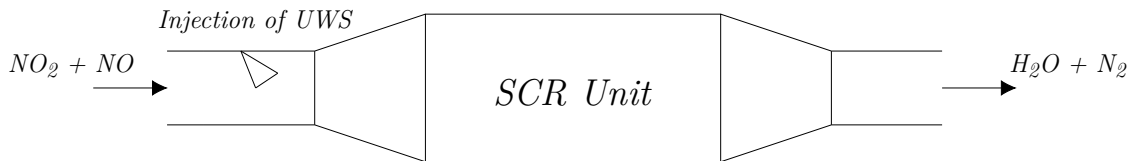
Figure 1.1: Simple schematic illustrating the principle of an SCR unit.
