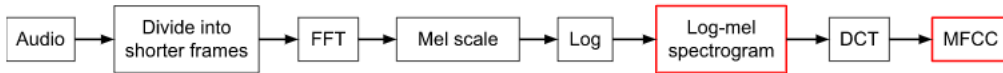
Figure 2.6: A flow chart describing the algorithm for extracting log-mel spectrograms and MFCC.
