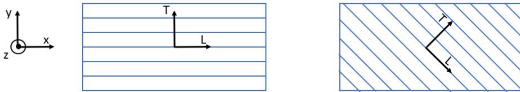
Figure 2.1: The coordinates in an lamina with respect to the fibre where z -direction points outwards from the lamina.
