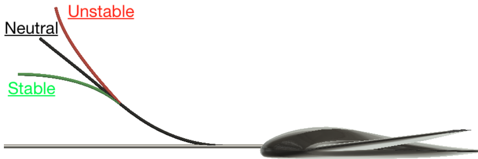
(a) Aircraft that is either pitch stable, neutral or unstable
