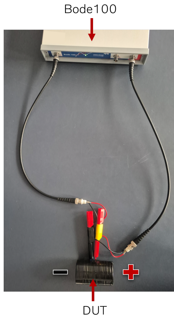
Figure 4.22: Cylindrical cell measurement setup
