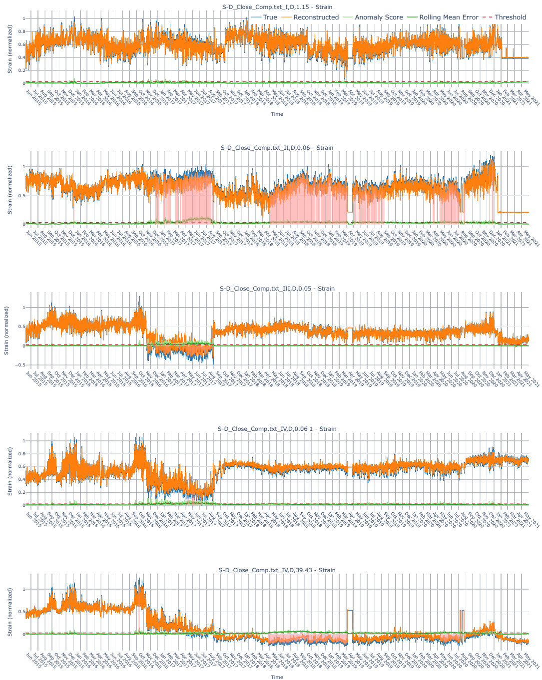
Figure A.3: True vs. predicted signal for the test data for S-D_Close_Comp at support I-V.
