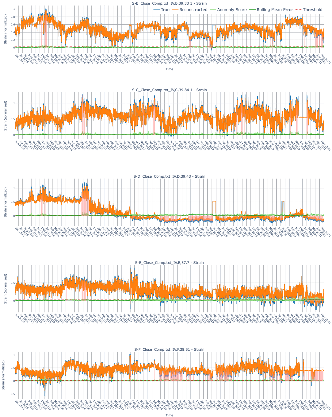
Figure A.10: True vs. predicted signal for the test data for beam B-F at support V.
