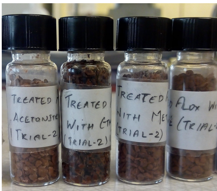
Figure 4.1: Regenerated Samples from Soxhlet Extraction: (from the left) a. Acetonitrile b. Ethyl acetate c. Methanol d. Acetone
