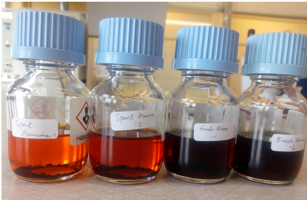
Figure 4.13: Used and Fresh alumina (double sample) after aluminum oxide performance test
