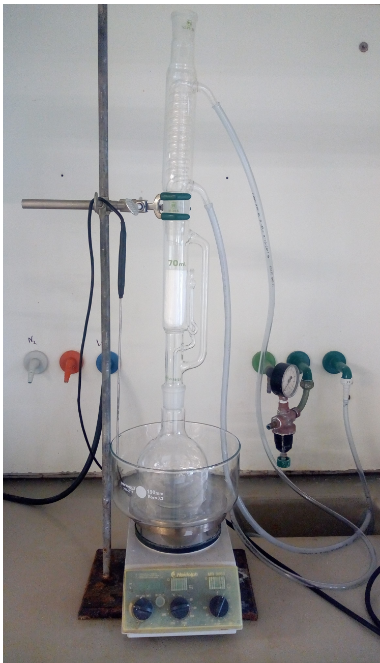
Figure 2.13: Lab set-up of Soxhlet extractor
