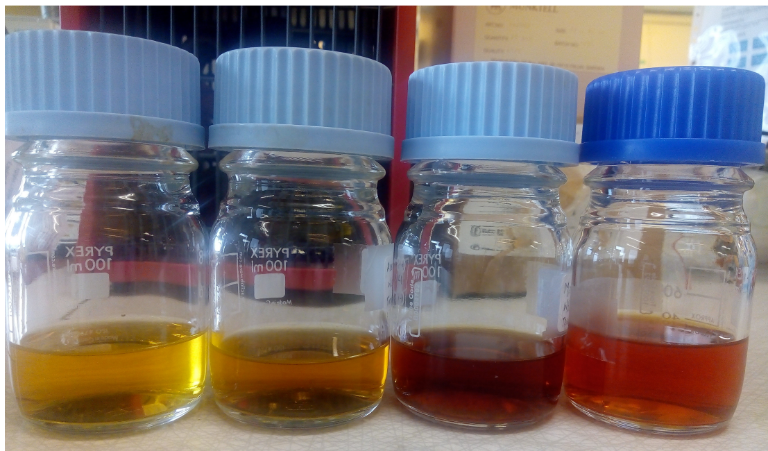
Figure 4.2: Extraction solvent after the Soxhlet extraction (from the left) Acetone, Acetonitrile, Ethyl acetate and Methanol
