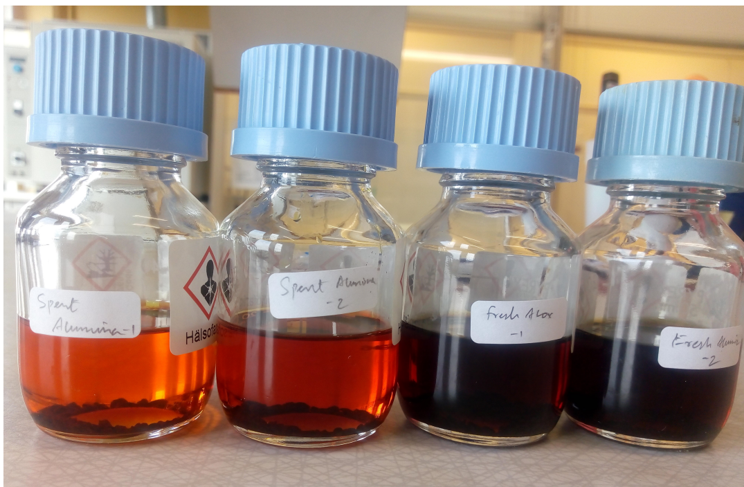
Figure 3.1: Sample mixtures of Fresh and used alumina immersed in standard epoxide solution
