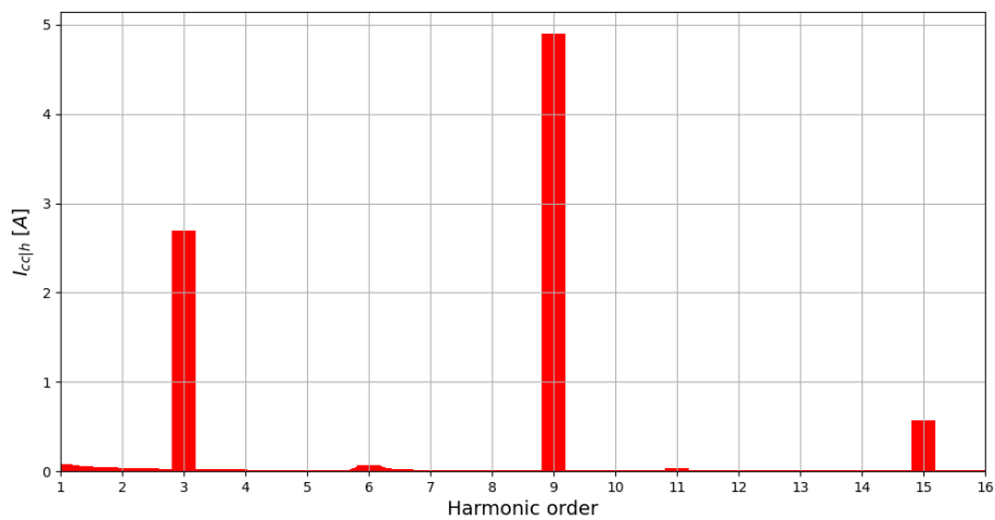
Figure 5.7: I_{cc} in no-load at 3000rpm
