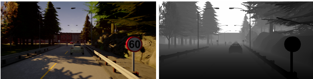
Figure 3.1: Example of a RGB and depth image of a simulated traffic environment in Carla.
