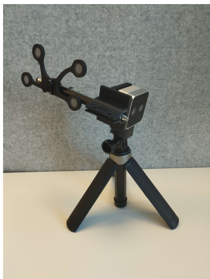
(a) The Intel® RealSense™ D405 fitted with a custom 3D printed mount along with a navigation system marker .
