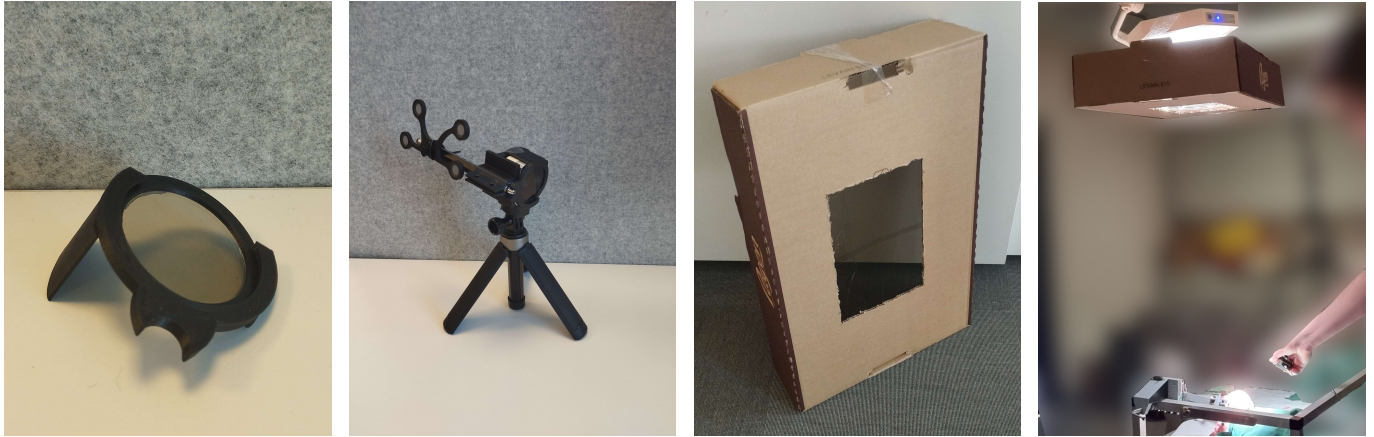
(a) Custom 3D printed polarisation filter, attachable to the depth camera. (b) The Intel® RealSense™ D405 depth camera fitted with a custom 3D printed mount along with a navigation system marker. (c) A box with a hole fitted with polarisation filters, used to filter the surgical spotlight. (d) Light source polarisation filter mounted to the surgical spotlight.
