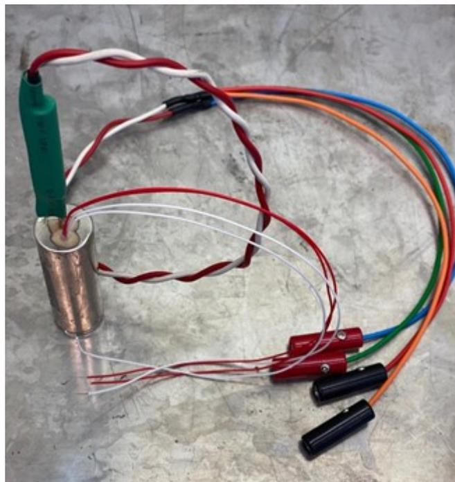
**Figure 7.8:** Drilled cell both the temperature sensor and the heater installed.
