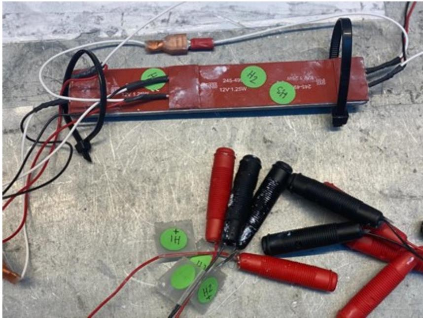
**Figure 5.3:** First heater utilized in the axial thermal conductivity experiments.
