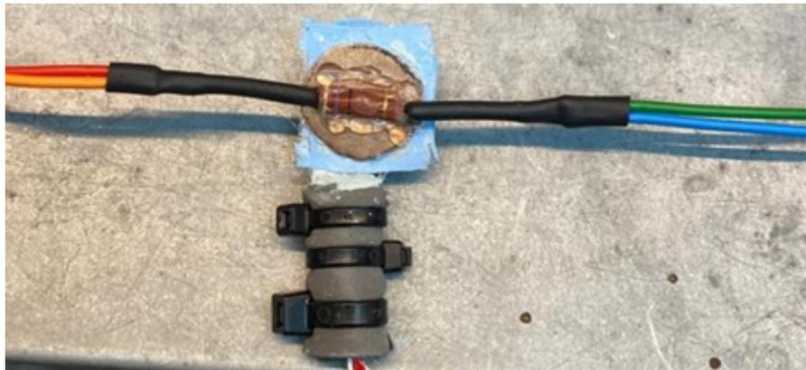
**Figure 5.4:** Second heater utilized in the axial thermal conductivity experiments.
