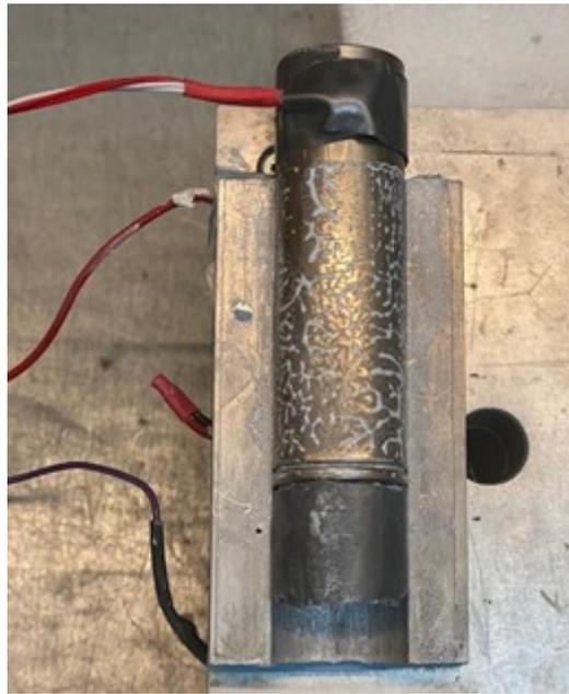
**Figure 7.4:** Additional temperature sensor attached to the cell's surface.
