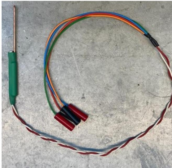
**Figure 7.7:** Heater utilized in the measurements of the cell's radial thermal conductivity.
