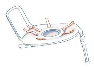
*Figure 23. Ducts through the base to prevent gathering of dirt between the base and the seat.*
