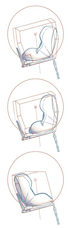
*Figure 24. Size constraints, rotation sphere and rotation axis of the seat.*
