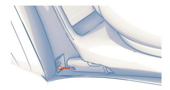
Figure 2. ISOFIX connectors and anchor points.
