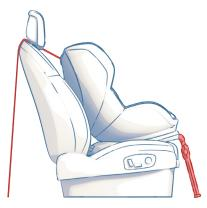
*Figure 15. Top tether strap and support leg.*
