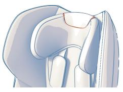
*Figure 19. Headrest height adjusted by operating the lever placed in the top.*
