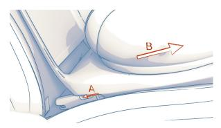
Figure 8. The button on the ISOFIX connector is first pushed to release it from the anchor point, after which force is applied to the connector in the opposite direction.
