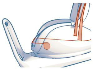
*Figure 22. Spool for gathering excess tensioning belt.*
