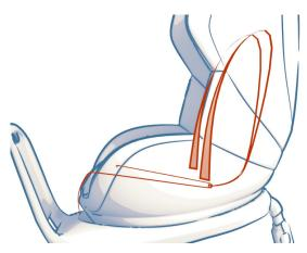
*Figure 21. Mechanical advantage harness system.*
