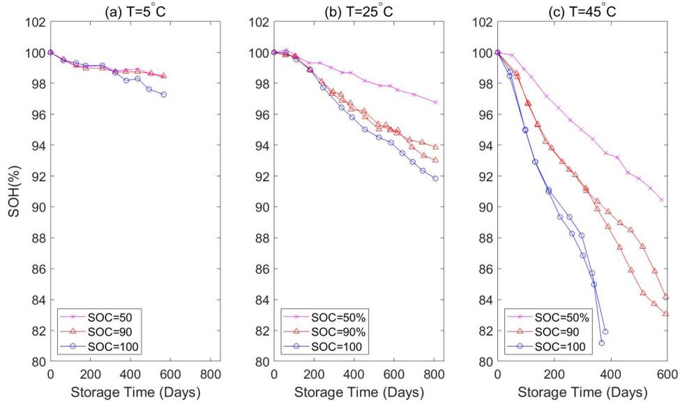
**Figure A.4:** Kokam Calendar aging data under testing temperature of 5, 25, 45 degree
