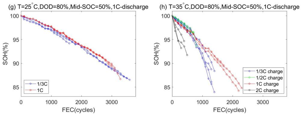
Figure A.8: Cycling test raw data in Battery2020
