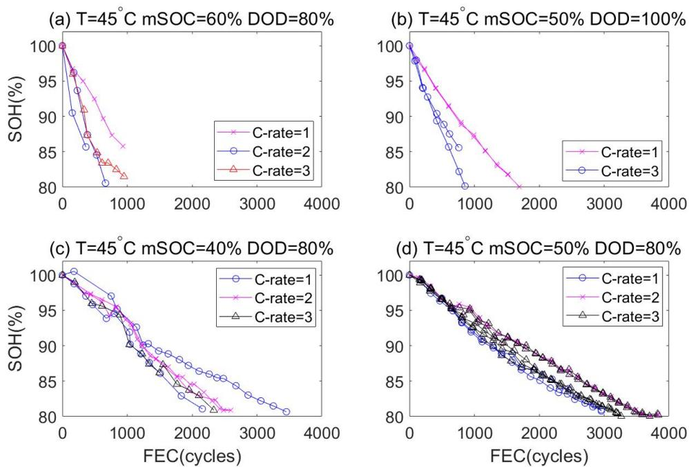
Figure A.10: Cycling test raw data of the Kokam cell
