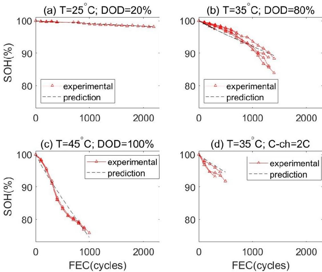
Figure 5.6: Cycling Modelling performance in project battery 2020
