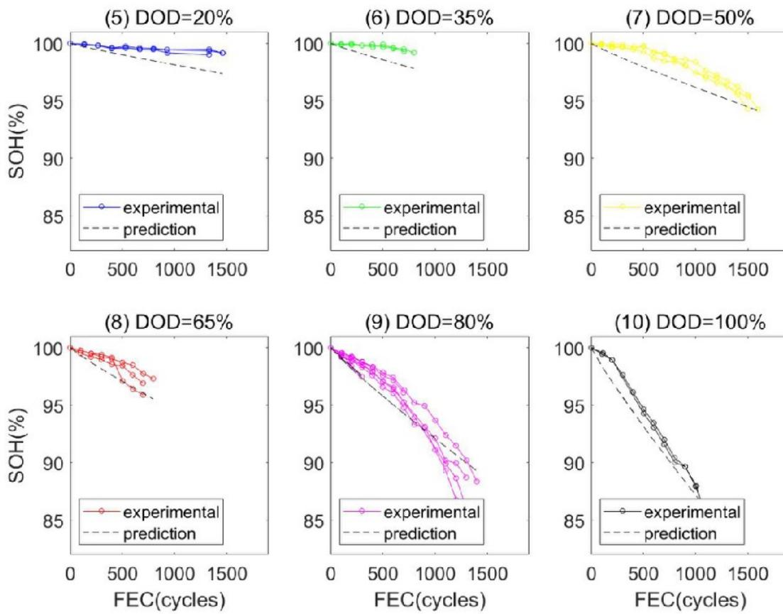
**Figure A.18:** Cycling modelling predicted performance of the cells in Project Battery 2020
