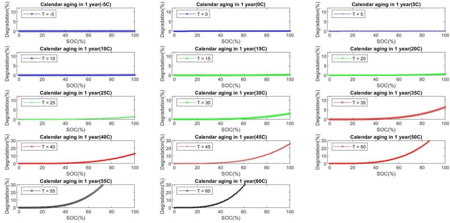
Figure A.15: Battery degradation in one year in different storage temperatures
