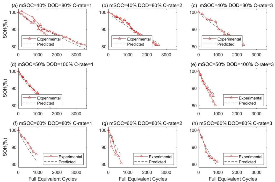
Figure A.22: Cycling modelling predicted performance of the Kokam cells
