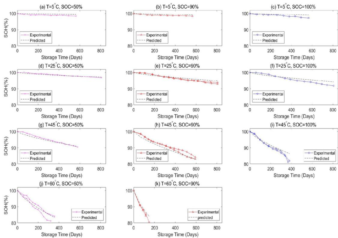
**Figure A.12:** Cycling modelling predicted performance of the cells in Project Mat4Bat
