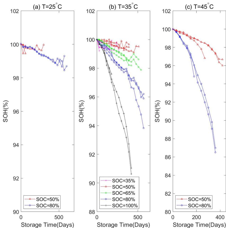
**Figure 4.1:** Calendar ageing data in battery2020 project.(a)Temperature = 25°C; (b)Temperature = 35°C; (c)Temperature = 45°C
