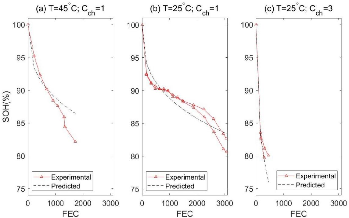
**Figure 5.8:** Cycling Modelling performance of the Kokam cells in project Mat4Bat
