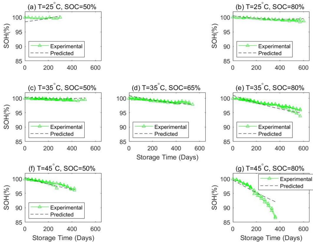
**Figure 5.1:** Linear model(Battery 2020 project data set: calendar ageing)
