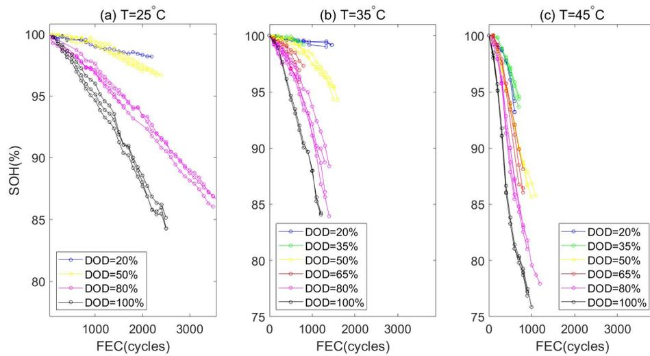
**Figure A.5:** Kokam Calendar aging data under testing temperature of 5, 25, 45 degree
