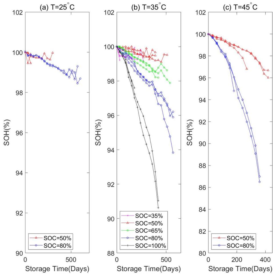
**Figure A.1:** Calendar aging data in battery2020 project. (a) Temperature =  $25^{\circ}\text{C}$ ; (b) Temperature =  $35^{\circ}\text{C}$ ; (c) Temperature =  $45^{\circ}\text{C}$
