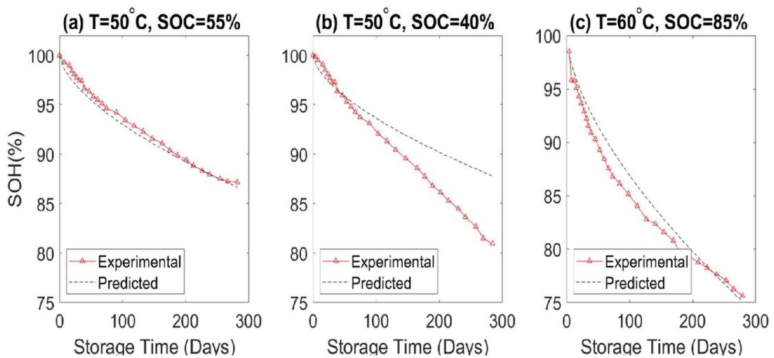
**Figure A.14:** Calendar modelling predicted performance of the LBG cells in Other temperature
