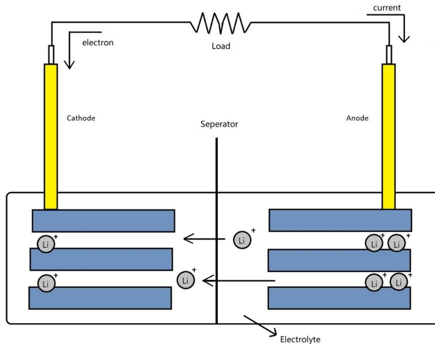
**Figure 2.1:** The electro-chemical reactions in Lithium-ion battery
