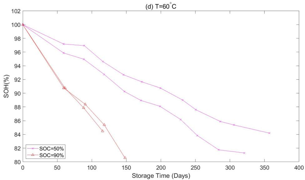
**Figure A.3:** Kokam Calendar aging data under testing temperature of 60 degree
