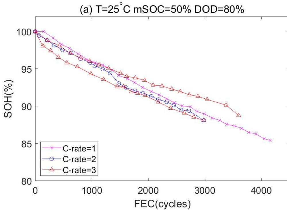
Figure A.9: Cycling test raw data of the Kokam cell
