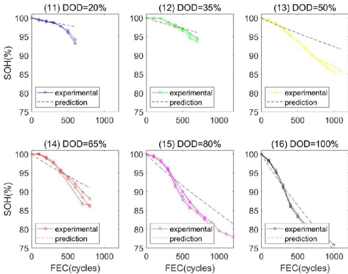
**Figure A.19:** Cycling modelling predicted performance of the cells in Project Battery 2020
