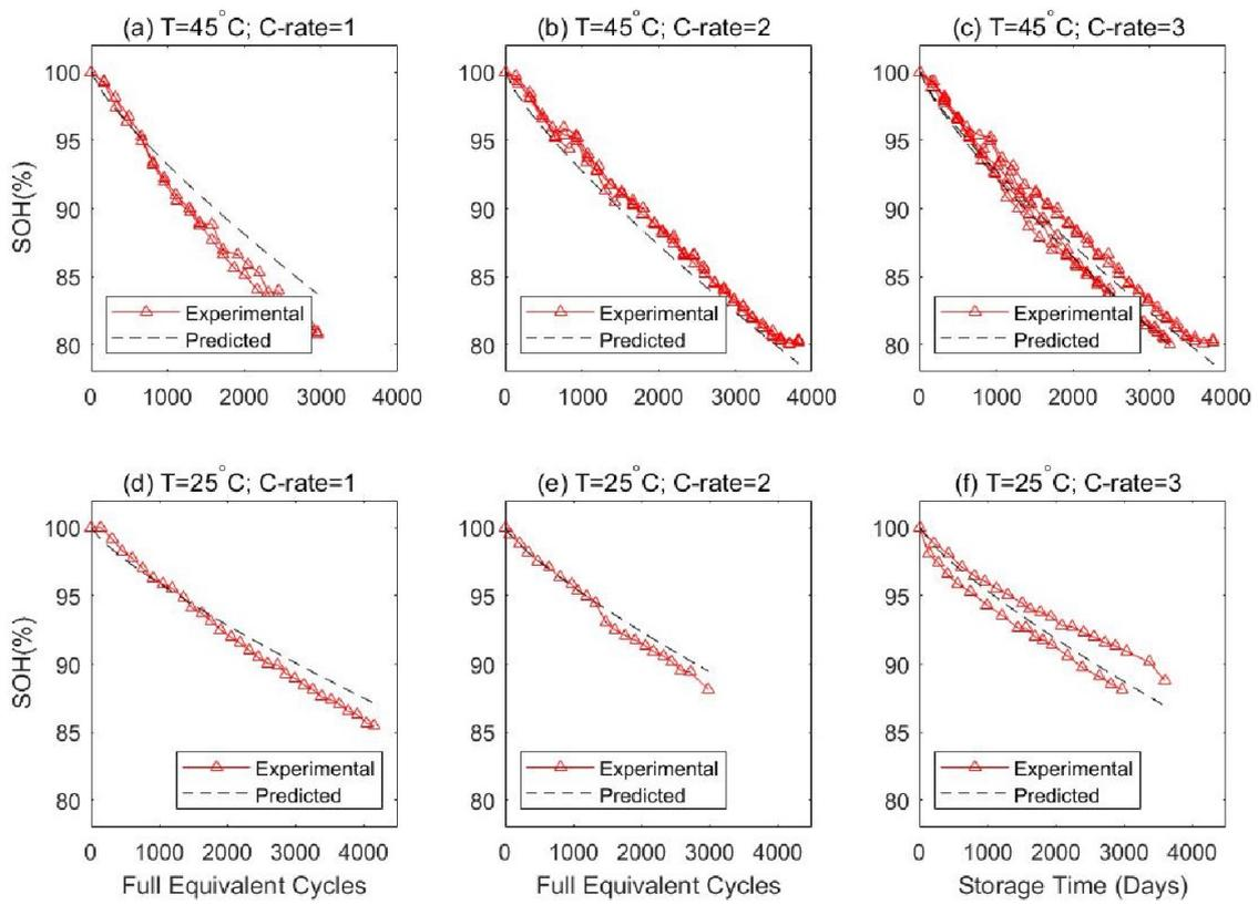
**Figure A.23:** Cycling modelling predicted performance of the generated cells
