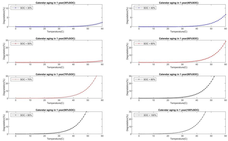
Figure A.16: Battery degradation in one year in different storage SOC levels
