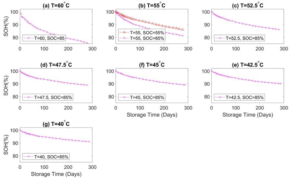
**Figure A.2:** Calendar aging data of the LGB cells under other temperature conditions
