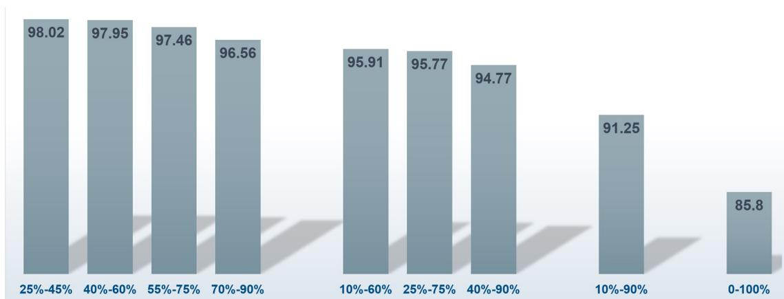
**Figure 5.9:** State of Health (SOH) after 1000 cycles under different SOC-window
