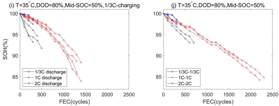
Figure A.7: Cycling test raw data in Battery2020
