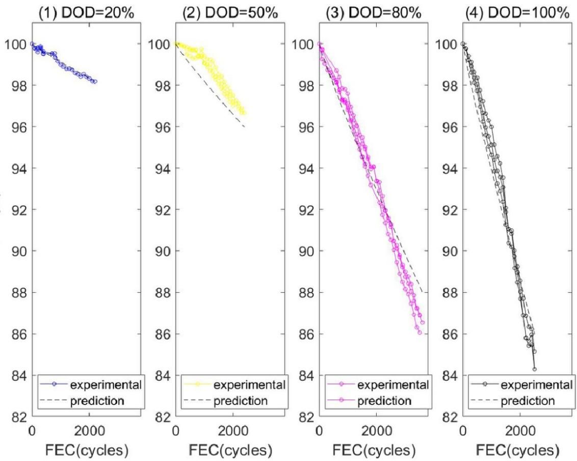
**Figure A.17:** Cycling modelling predicted performance of the cells in Project Battery 2020
