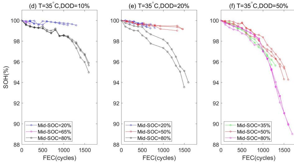
Figure A.6: Cycling test raw data in Battery2020
