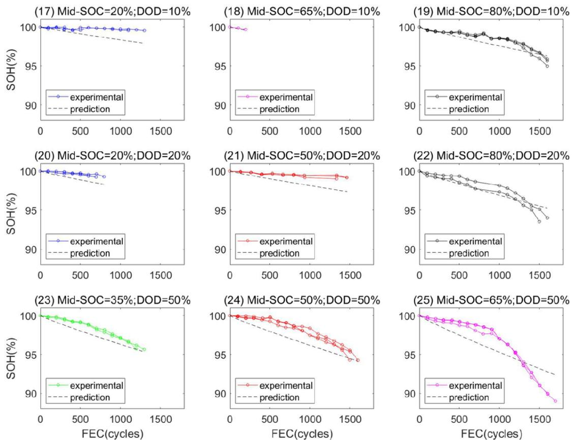
**Figure A.20:** Cycling modelling predicted performance of the cells in Project Battery 2020
