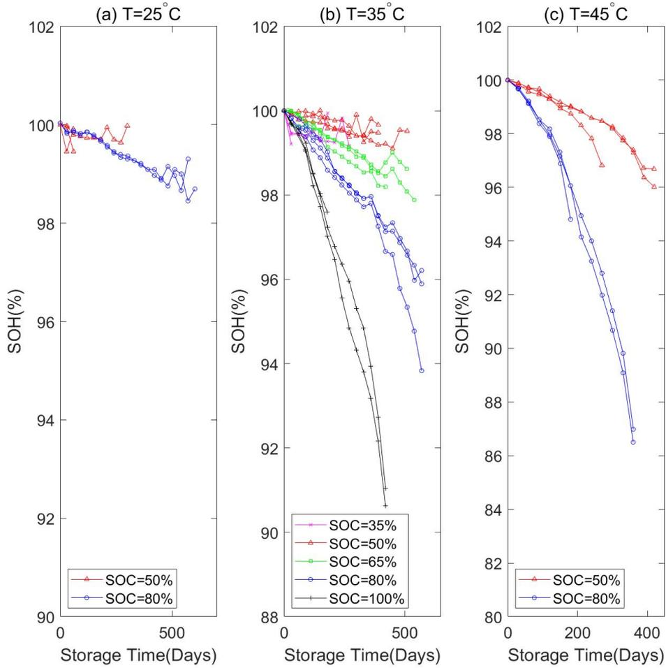
**Figure 3.1:** Calendar ageing data in battery2020 project. (a) Temperature = 25°C; (b) Temperature = 35°C; (c) Temperature = 45°C
