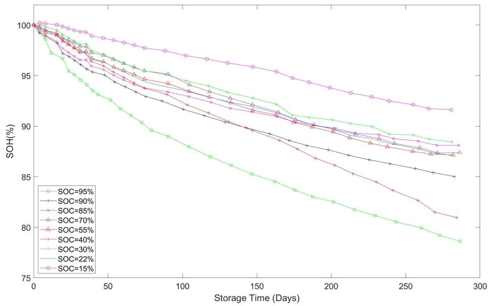
**Figure 3.2:** Calendar ageing data of LBG cells when the testing temperature is 50 degree
