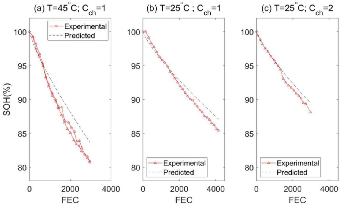
**Figure 5.7:** Cycling Modelling performance of the Generated cells in project Mat4Bat
