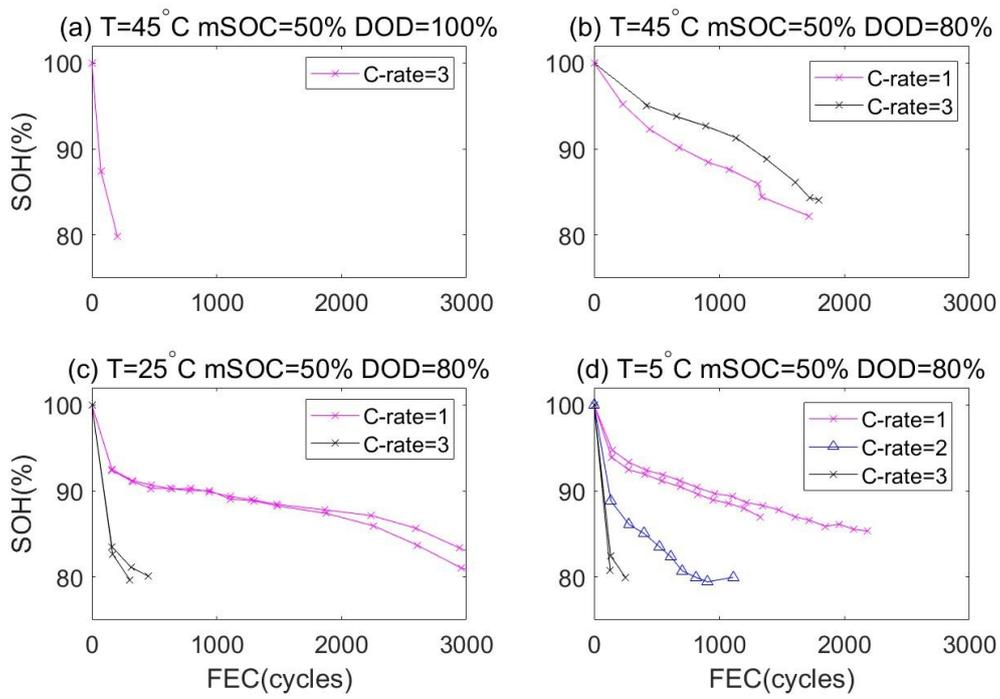
**Figure A.11:** Cycling test raw data of the generation cell in Project Mat4Bat
