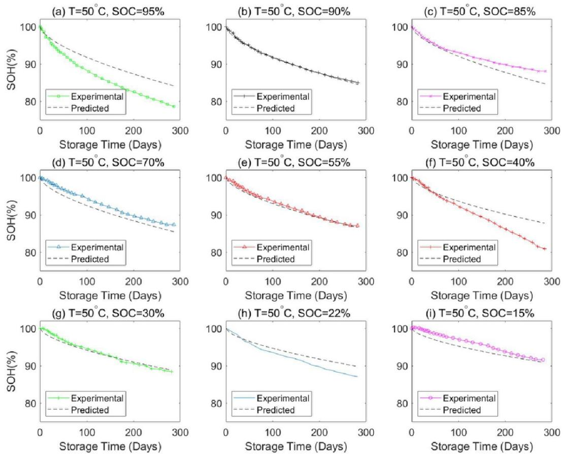
**Figure A.13:** Calendar modelling predicted performance of the LBG cells in 50 degree
