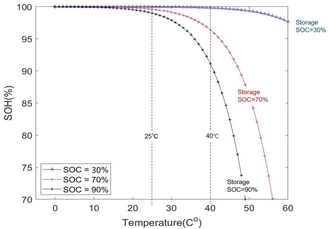
**Figure 5.5:** State of Health (SOH) after storageing 1 year under different SOC
