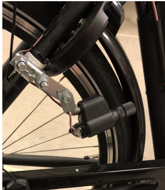
Figure 2.14: DC motor placed inside the bike's dynamo and used as speed sensor
