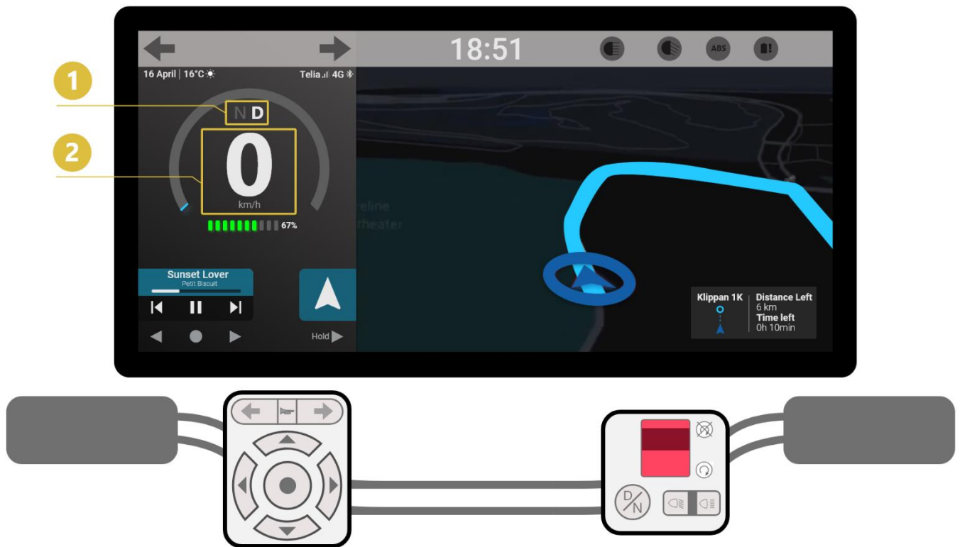
Figure 47. Dashboard changes when Drive mode is initiated. The rider no longer has access to quick menu and can no longer interact via the touch display.
