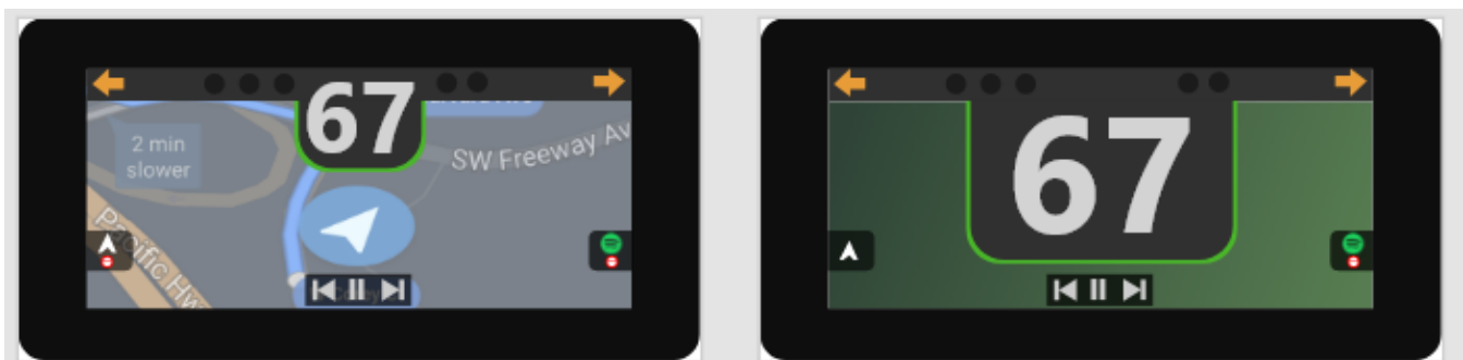
Figure 29. Showing an early stage prototype where the speedometer would adjust to what was active. This was later stripped down and made simpler as it was realized that essential elements for riding should not move around.
