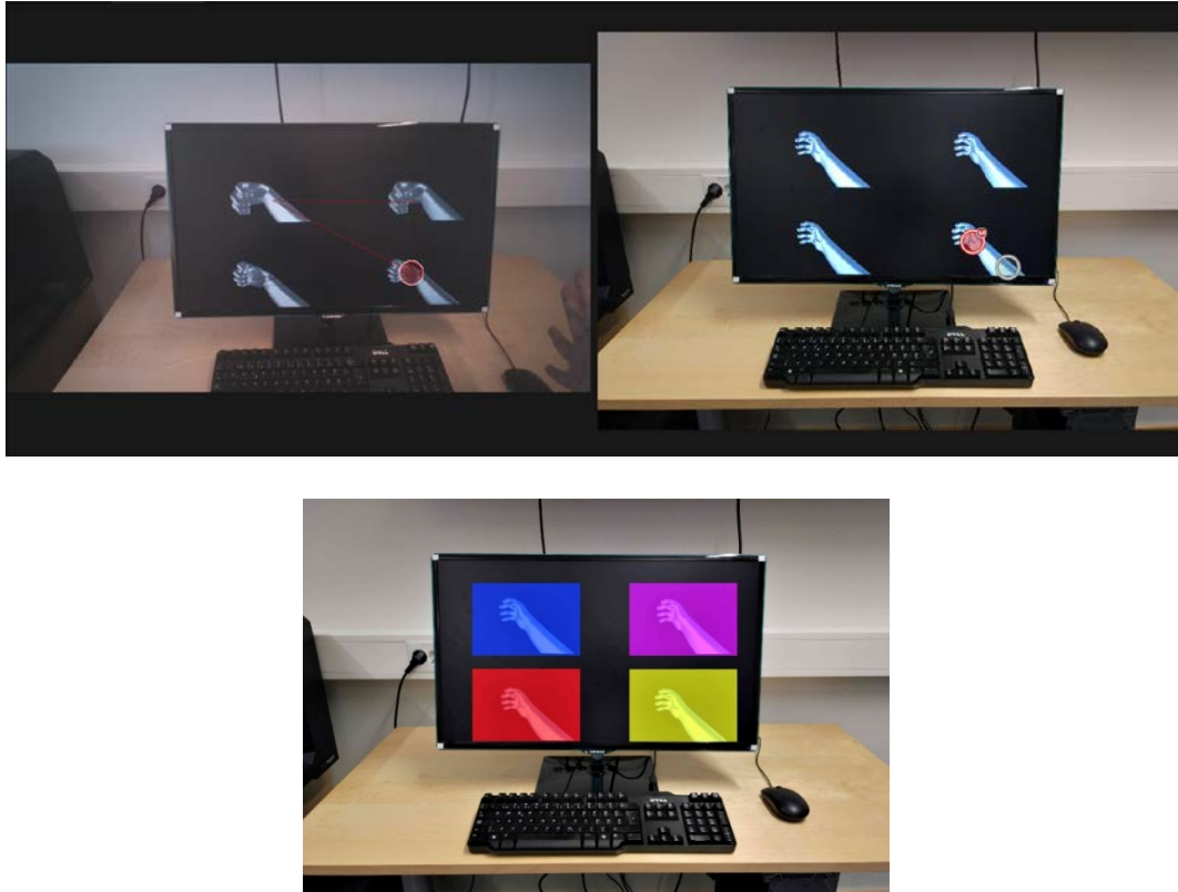
Figure 14. Snapshot from the user interface in Tobii Pro Lab software showing a red circle denoting the recorded gaze point on a single frame in the scene-camera recording of the wearable eye-tracker (left), and the reference image on which gaze points from the recording were mapped onto (right). Furthermore, the gray circle shows the software's attempt at automatically mapping the gaze point, and the red circle with the letter M in its border was the manual remapping of the gaze point with a point and click of a mouse. Four equal-sized rectangular areas of interest (bottom) were placed symmetrically around each VR arm in a quadrant to classify whether an eye-fixation was located on a virtual limb or not.
