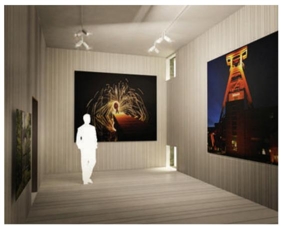
One of the large exhibition spaces, the windows in this room corresponds to the existing windows in the exterior skin. The placement towards the floor and the ceiling give a soft light and the absence from views to the void and the exterior gives full focus to the exhibited items
