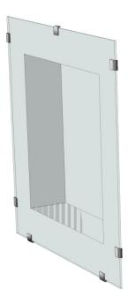
In order to make the concrete shell wind and rain tight the existing openings need to be sealed whether they are old windows or holes due to the decay of the building. A simple plane of glass is attached to the existing wall by metal clamps and the sealed with a soft joint.
