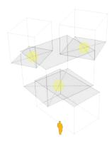
The center of gravity for each box is located on the box beneath.
