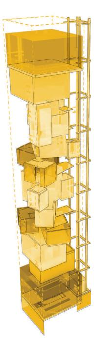
The program is arranged vertically. The movement through the building is done by the means of the elevator just as in a mine, but there are shortcuts with ladders and climbing nets that the visitors can use to move from one function to the other.
