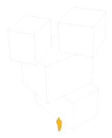
The structural system are made up by stiff frame boxes made from steal profiles. The boxes are then stacked on top of each other
