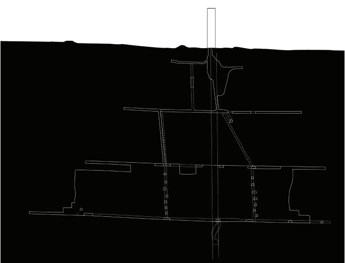
A sectional drawing of the mine, the underground spaces are an intricate system of shafts and drifts reaching all the way down to 260 meters of depth.
