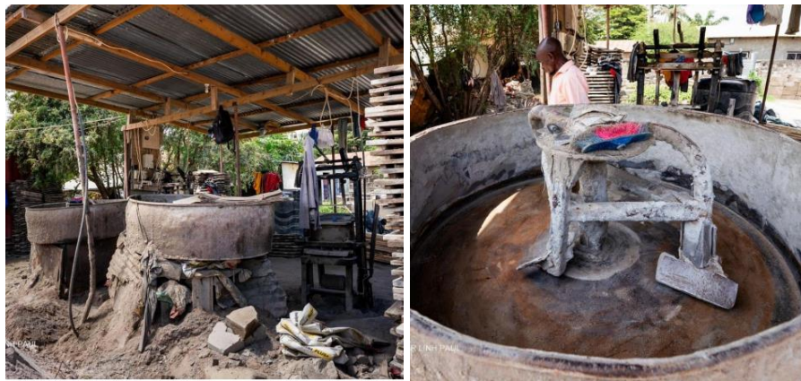
Figur 3 Befintlig panmixer. (Engineers Without Borders Sweden, Foto: Linh Paul).
