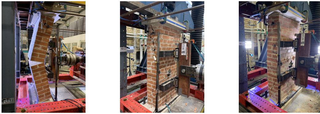
(a) Wall W5 with a bending failure. (b) Wall W12 with a shear failure. (c) Wall W14 with a bending/shear failure.
