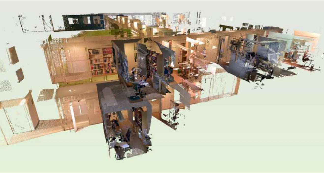
Figure 17. 3D scanning as a way of logging and storing inventory data, using White Recapture (White ReCapture n.d.).
