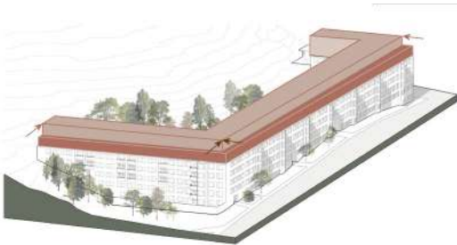
3. TOP STOREY RETRACTED ON STREET SIDE to minimize the height impression for walkers-by. Two meters retraction on long side and three meters on short sides.
