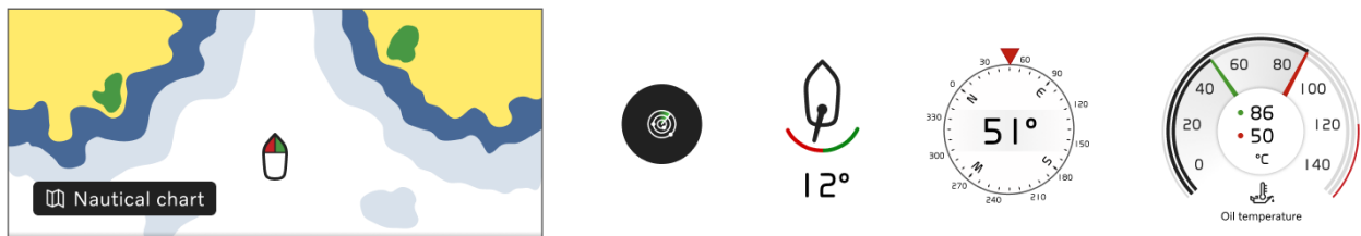
Figure 3. A selection of the user interface elements designed for the different display features, from left: nautical chart function, radar overlay shortcut, rudder angle, heading compass, and combined gauge for oil temperature.
