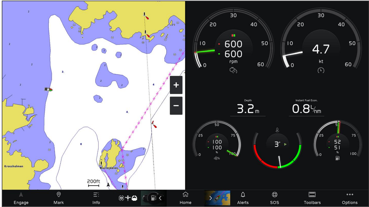
Figure 5. The interface for Glass Cockpit, displaying the nautical chart and engine data for a twin installation. 3
