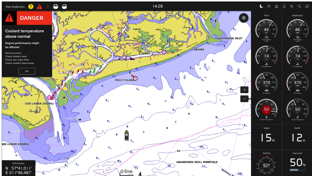
Figure 94. The final dark mode design for the Driving view with an alert pop-up.
