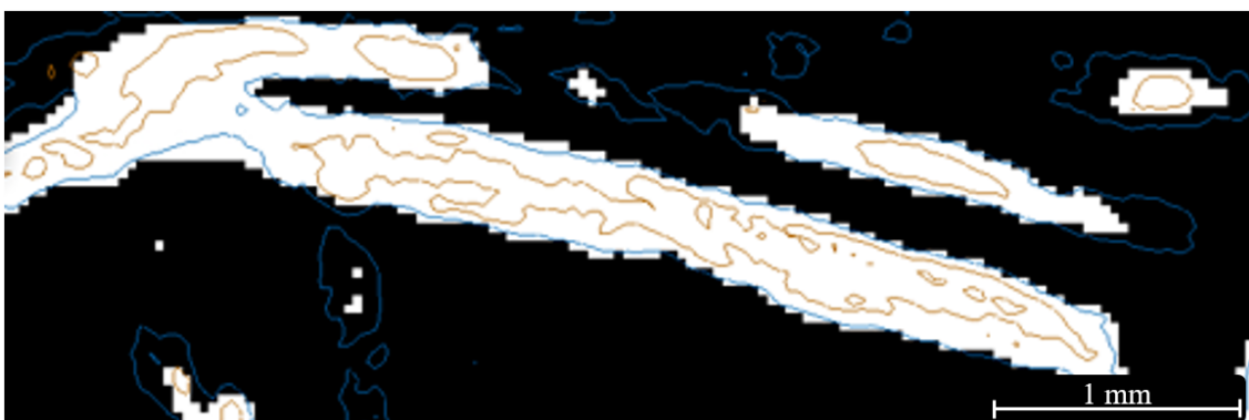
Figure 3.9: Image showing the fibre seed value (orange) and the fibre propagation value (blue). Black parts are void and matrix whereas the white parts are fibres, from RETOMO.
