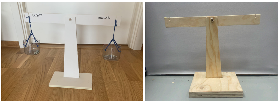
Figure 5: Balance scale mock-ups. The cardboard mock-up (left) and the mock-up in plywood (right).
