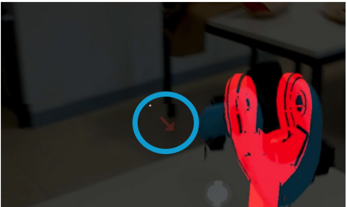
Figure 2.5: A virtual red arrow marked in the blue circle is used to capture technician's attention by pointing to the direction of the fault
