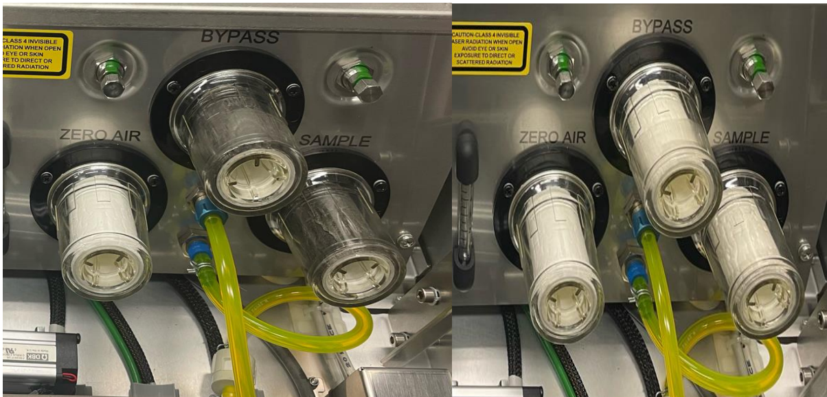
Figure 23b: The filter with capture soot to the left photo vs the cleanly filter the right photo.
