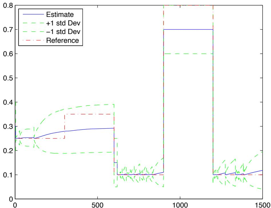
**Figure 6.1:** Simulation with road surface information and measurements at 100% tire-force utilization
