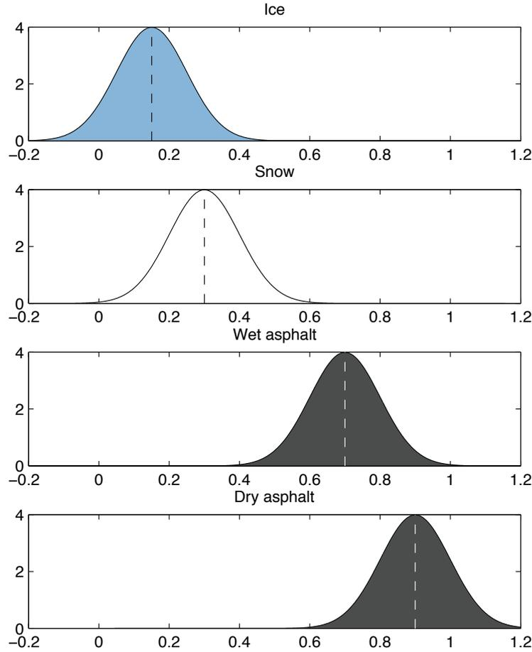
**Figure 3.1:** *Priori* distributions for ice, snow, wet asphalt and dry asphalt
