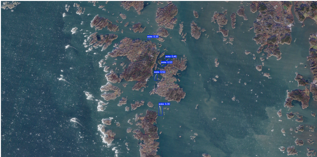
Figure 5.4: Wake detection with strong sea-surface clutter, breaking waves, coastlines, and visible background texture.
