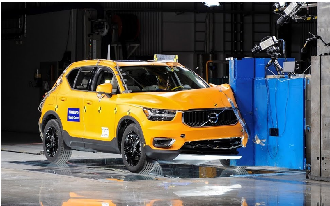
Figure 3: Overlap crash test XC40 [6]
