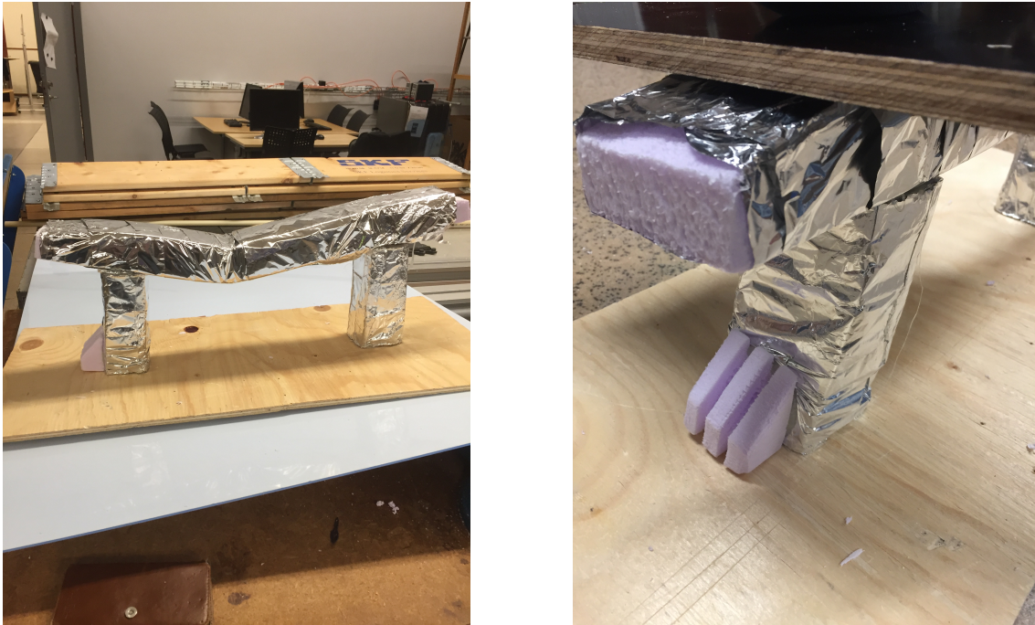
Figure 38: The bent bumper beam (left) and the wrinkled crashbox (right)
