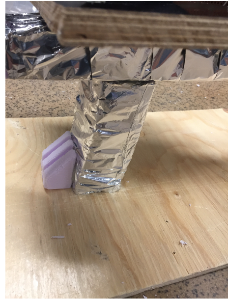
Figure 39: The failure of the CMS (left) and the wrinkled crashbox (right)
