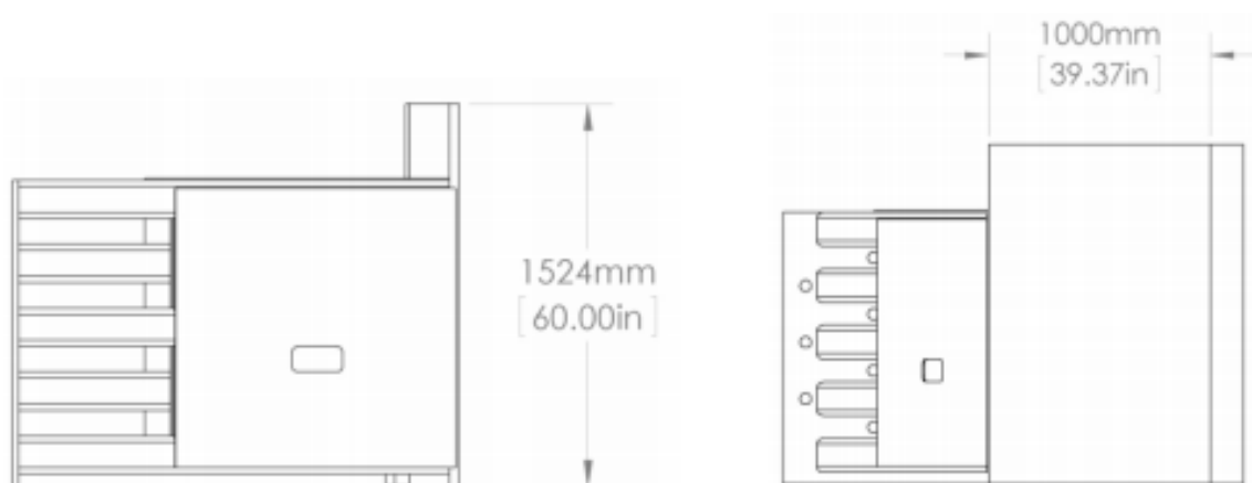
Figure 56: Profile view of small crash barrier
