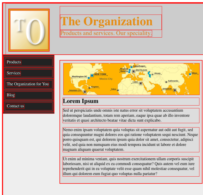
Figure 4. Each element is made visible by applying a red border to it, revealing the box model of this web page. Wherever the lines seem thicker, the borders of multiple elements are displayed. The web page is the same as displayed in Figure 1.
