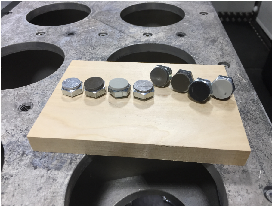
Figure 3.4: A display of different material inserts for both hammer and beam
