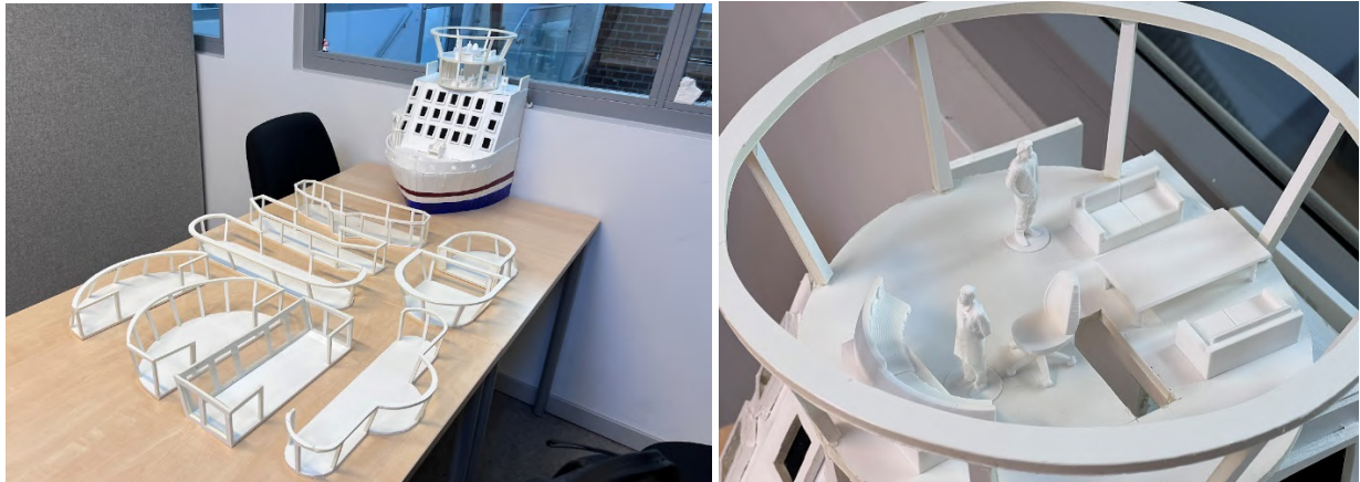
Figure 7: Physical ship model with interchangeable bridges and the 3D printed layout pieces.
