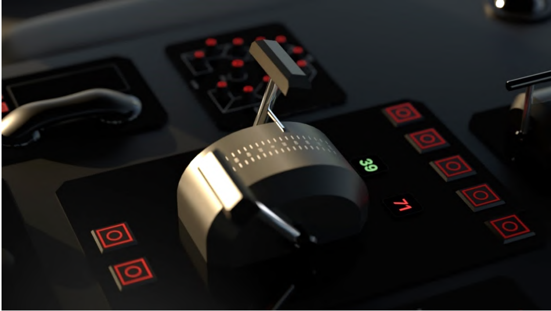
Figure 37: The main engine controls with indicators above.
