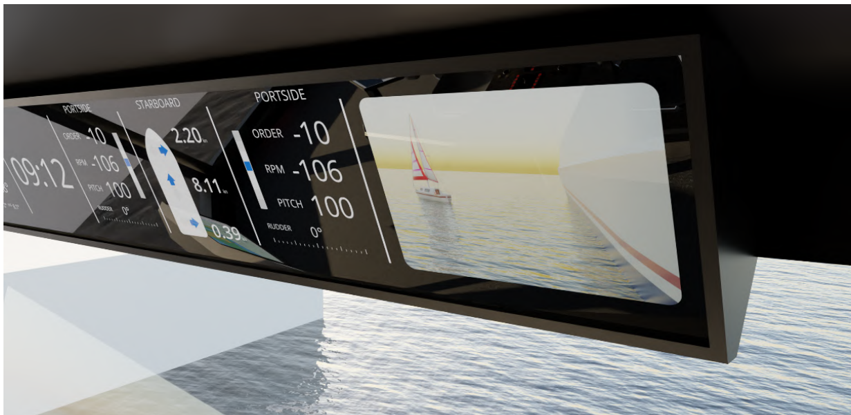
Figure 33: The starboard side camera view shown on the overhead display.
