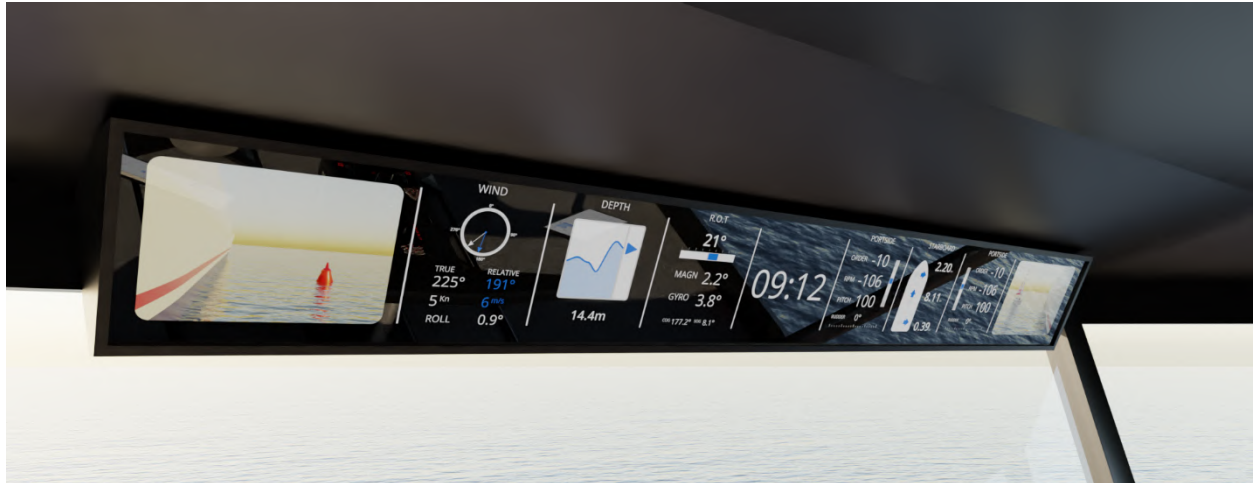
Figure 32: The overhead display with navigation information and live camera feeds.
