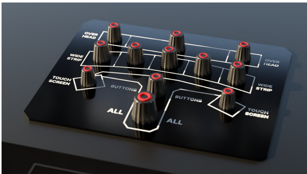
Figure 35: The dimming control hub.
