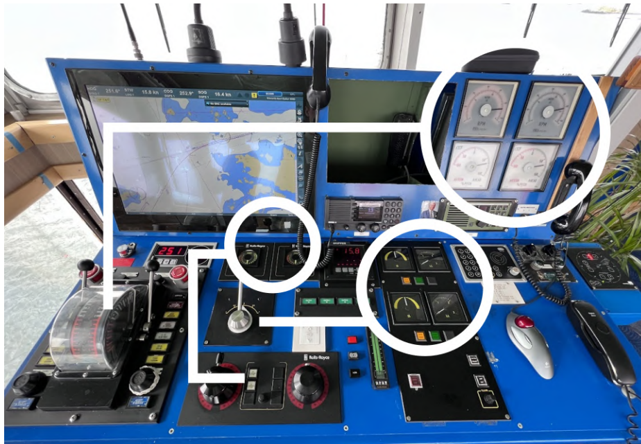
Figure 12: The unintuitive placements found on the wing bridge onboard Danica.
