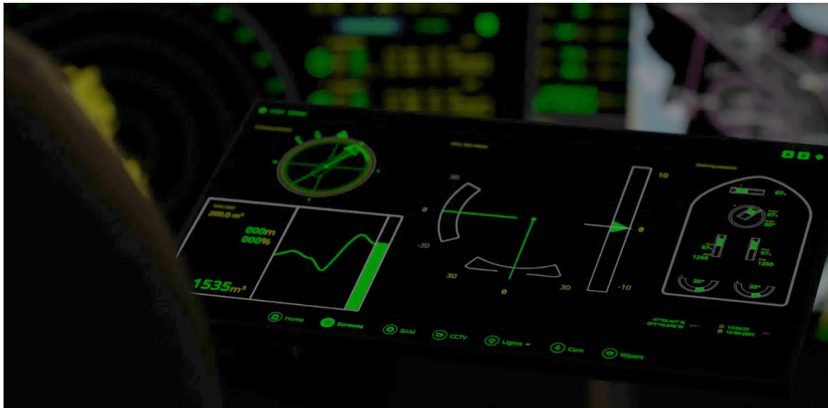
Figure 43: The inverted interface shown on the touchscreen, with the widestrip in the background.
